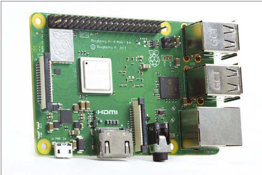
Figure 1: The new RPi3B+ meets some of the community's long-cherished needs, including faster wireless and Gigabit Ethernet (figure courtesy of the Raspberry Pi Foundation).
