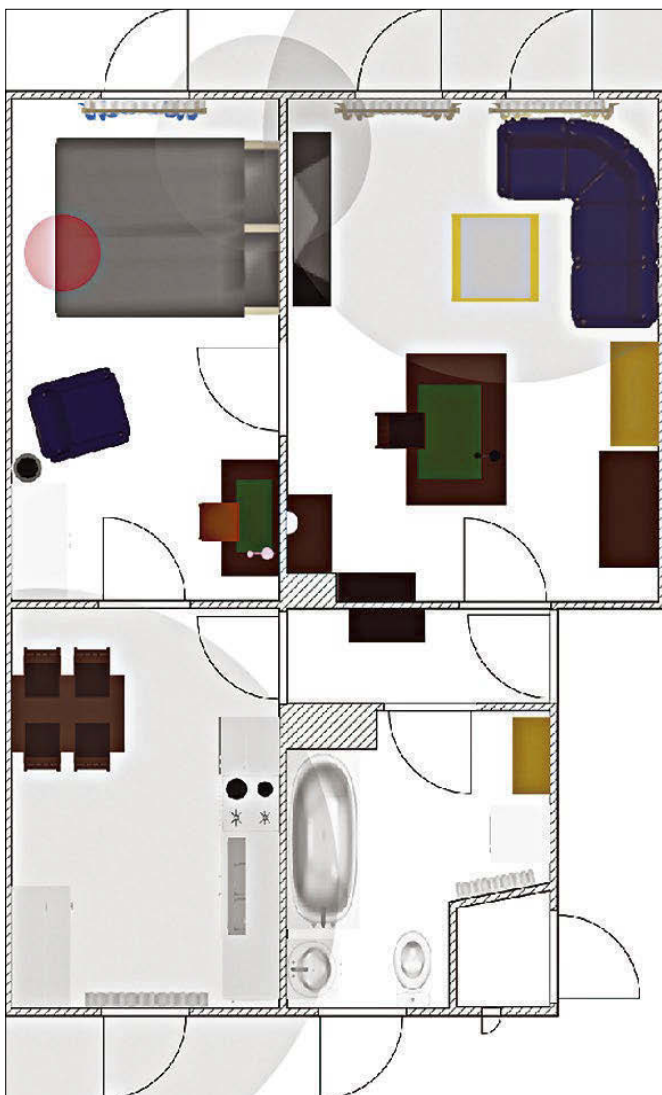
Figure 4: The room map shows the location of the Bluetooth beacon. The smaller the circle around the sensor, the closer the beacon is to the viewer.
