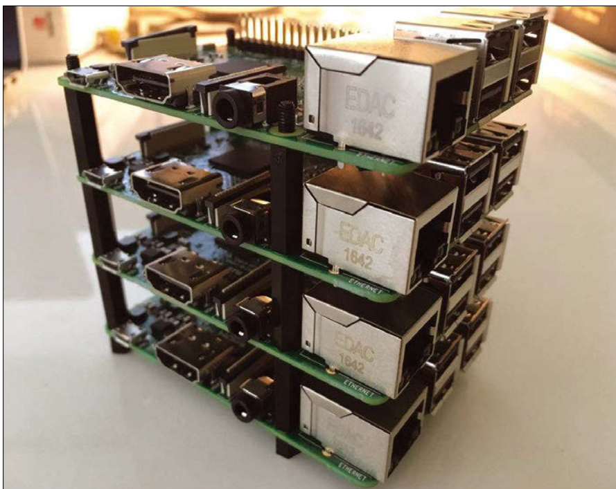
Figure 4: Raspberry Pis installed in a cluster. © howchoo.com
