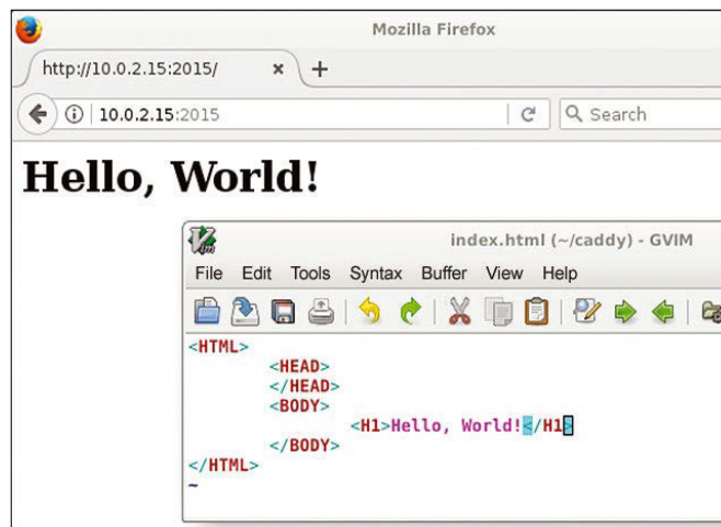
Figure 2: The website for the functionality test and the call in the web browser.
