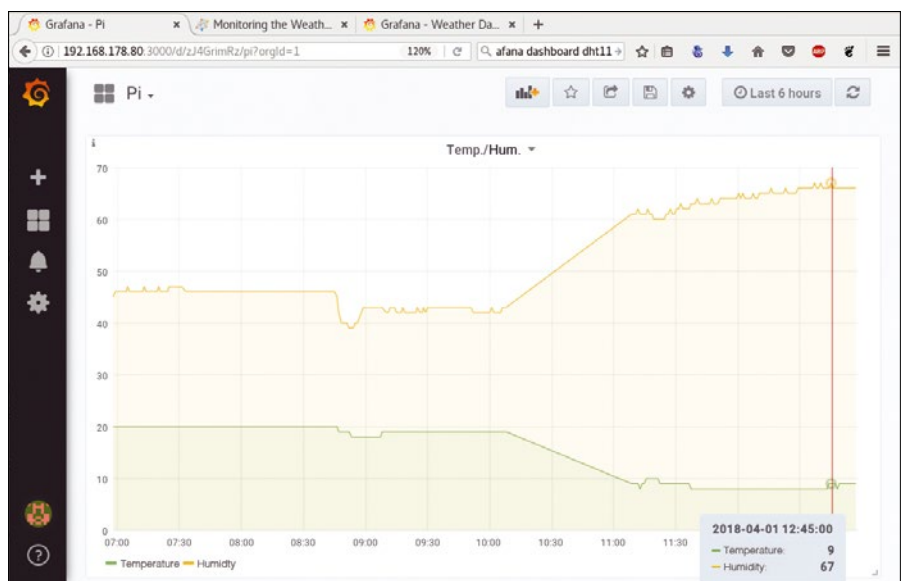
Figure 1: The sensor measures temperatures between 8°C and 9°C (ca. 46°F and 48°F) at the upper edge of the lower hive frame shortly after 10am, when the RPi2B was hung in the hive.
