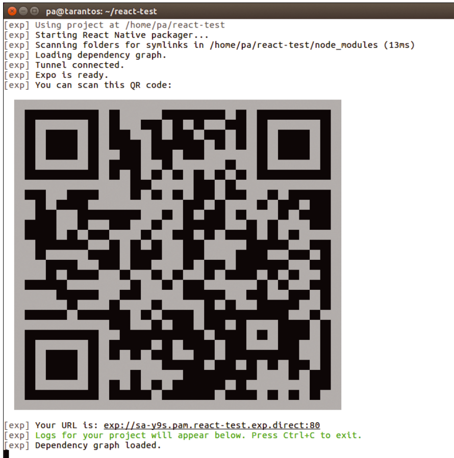
Figure 3: Expo offers the app for uploading in the Expo client like a website.
