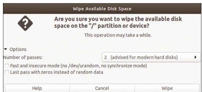
Figure 4: As a rule, it is sufficient to overwrite the data twice.
