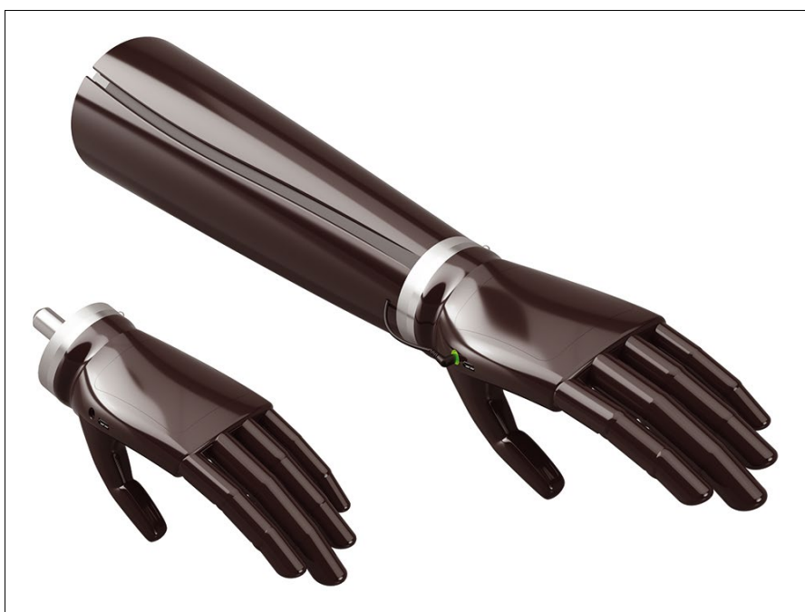
Figure 1: The development kit's artificial hand.
