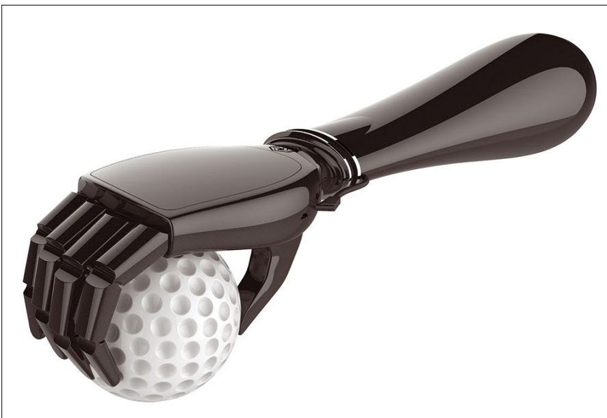
Figure 2: The Social Hardware hand will be capable of several different grips.
