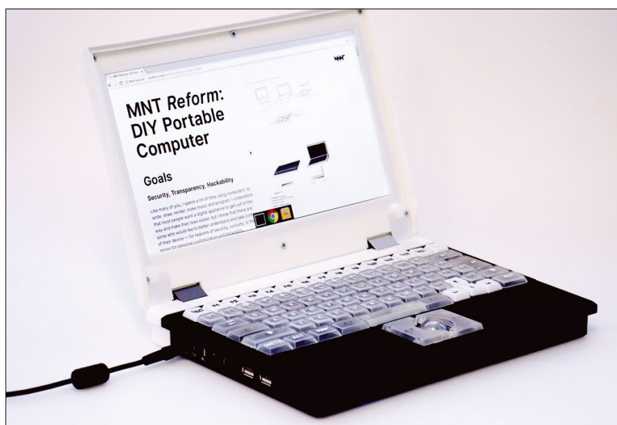
Figure 1: Reform is a modular, ergonomic open hardware laptop now in beta-testing.
