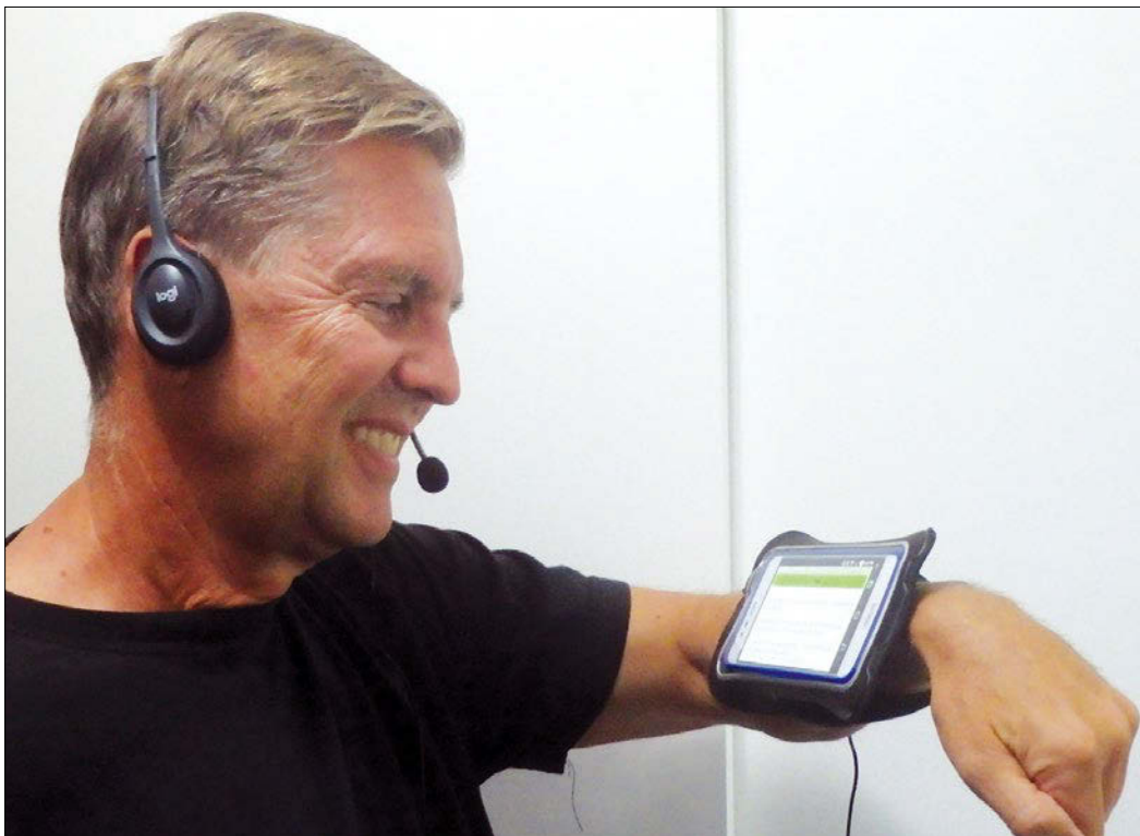
Figure 1: Hardware needed for this project: an Android smartphone mounted in an armband and headphones with a mic.
