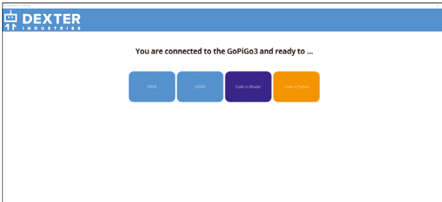
Figure 2: You program the robot in a web front end. The GoPiGo3 website takes you to the various programming environments and documentation.
