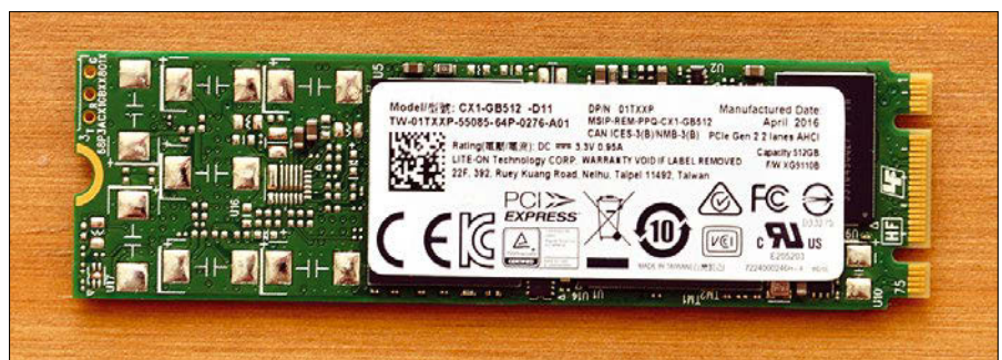
Figure 4: The Lite-On SSD complies with the PCIe AHCI standard.
