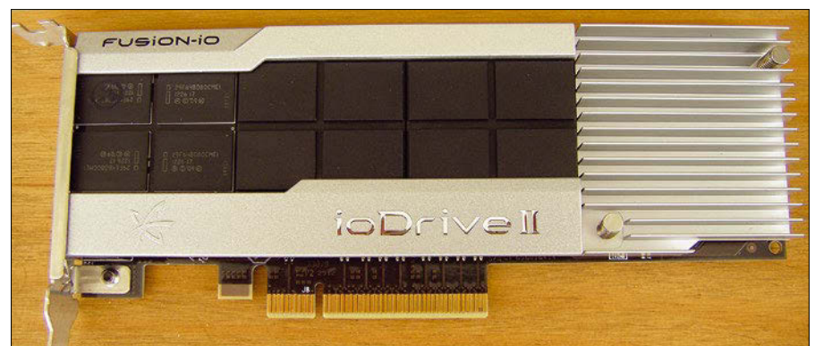
Figure 2: A PCIe SSD that can only be addressed with its own kernel driver on Linux.
