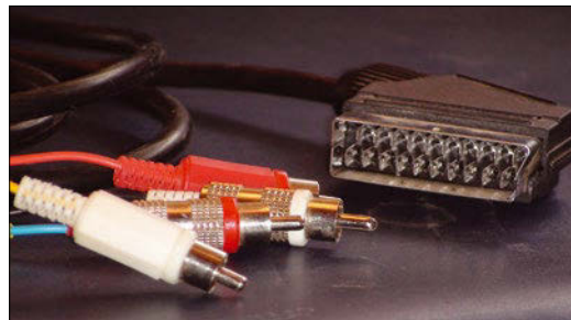
Figure 2: This SCART to RCA adaptor has an extra pin for audio input, which I won’t be using.
