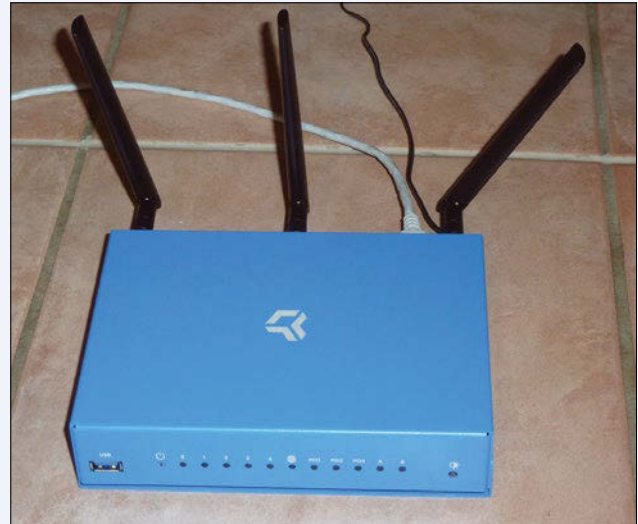
Figure 1: The open-hardware Omnia Turris from NIC.CZ saturates a GBit link without any problems.
