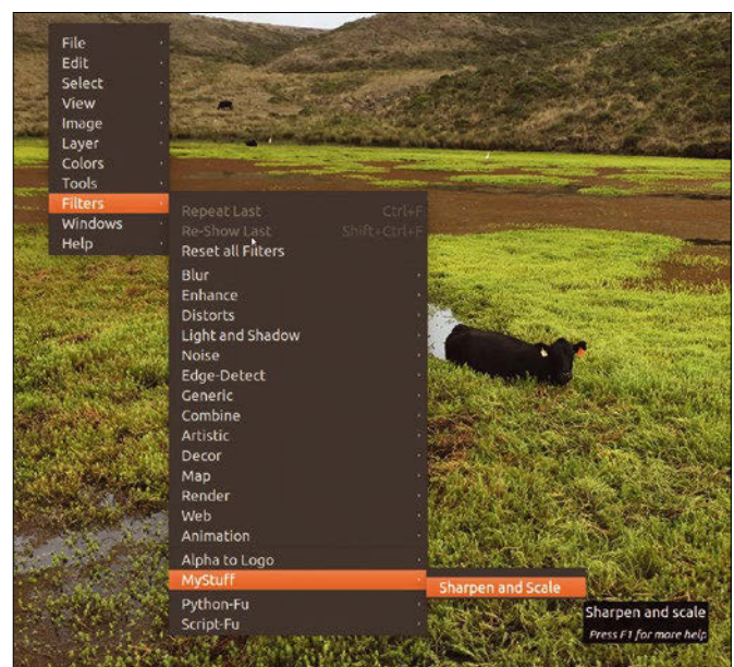
Figure 1: The menu entry for scaling and sharpening in Gimp, set up with a Python script.
