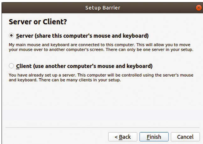
Figure 1: Barrier's initial setup wizard is used to configure the role of the system. The keyboard and mouse must be attached to the server.
