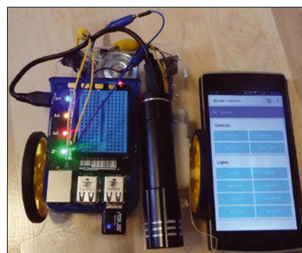
Figure 4: Raspberry Pi rover.
