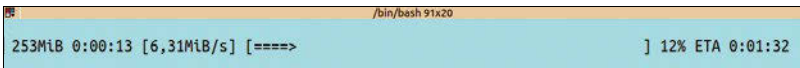
Figure 3: The pv program creates the most complete progress bars you can display in a Linux console.
