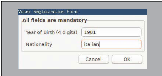
Figure 1: Who says that scripts are limited to command-line terminals? Use Zenity to make scripts create graphical forms.
