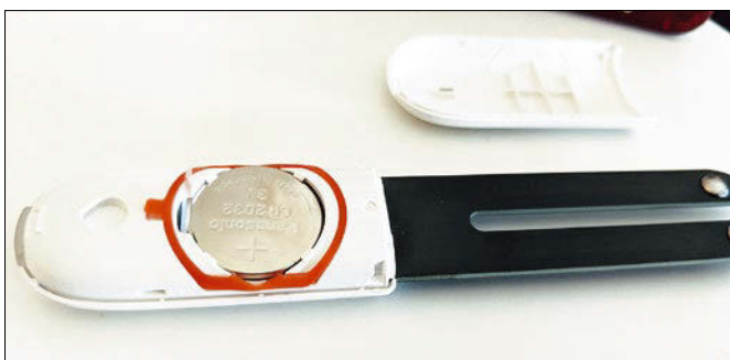
Figure 1: The Mi Flora sensor, which uses Bluetooth, is a spin-off product from the Chinese smartphone gadget market.
