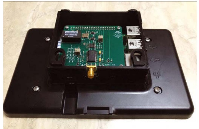
Figure 4: A modified Rasp Pi case allows the board's connector to protrude.
