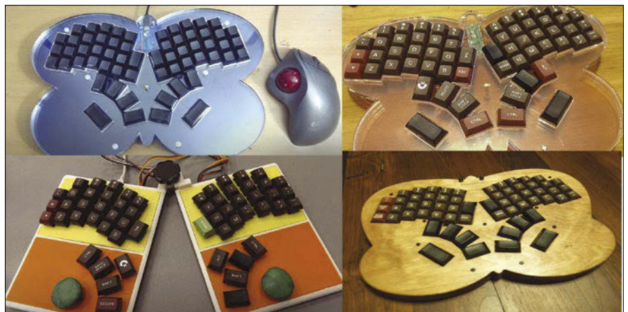
Figure 4: Some of the early prototypes for the Model 01.
