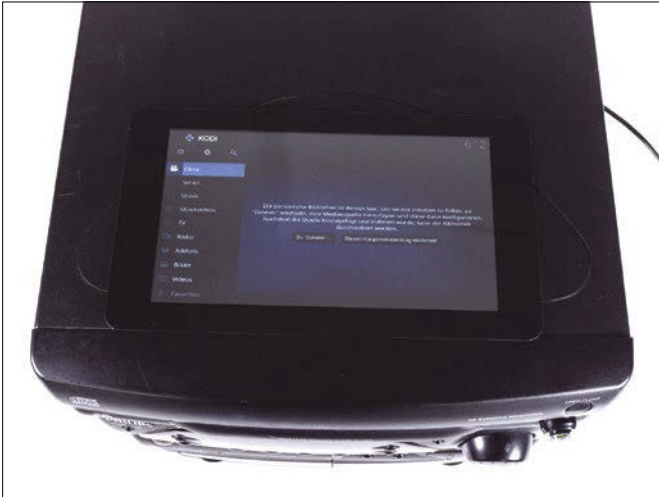
Figure 5: A seven-inch touch display and the Kodi media center make it relatively easy to browse a music collection.
