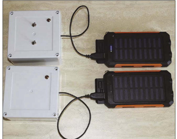
Figure 7: Switch and relay modules powered from solar-charged battery packs, ready for deployment.
