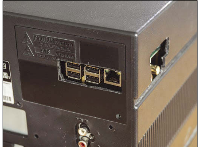
Figure 6: The Rasp Pi comes with at least four USB ports. It can be networked over the network drive and WiFi.
