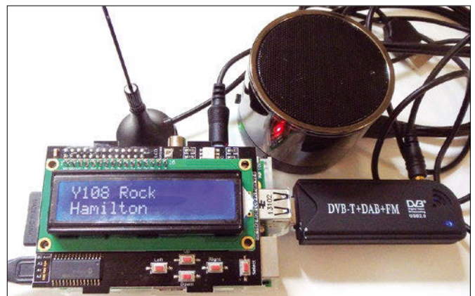
Figure 3: LCD keypad used on a Raspberry Pi FM radio project.
