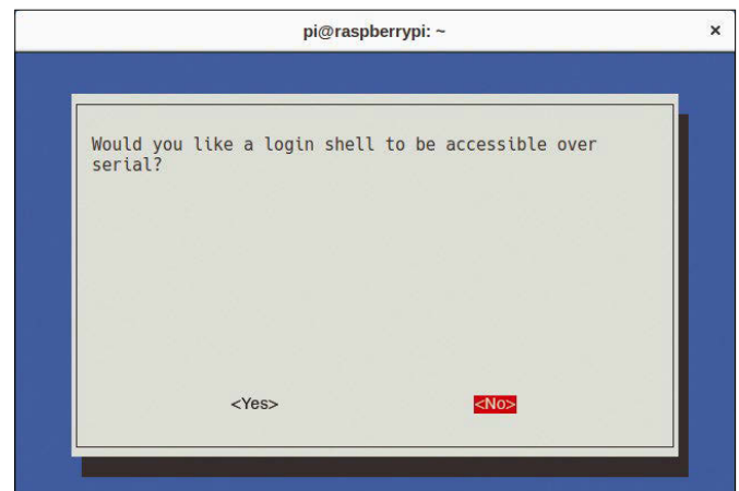
Figure 2: To enable FHEM to integrate the RaZberry module, you'll need to deactivate the terminal function of the serial interface.
