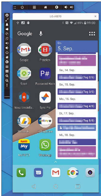
Figure 3: An Android smartphone screen on the Linux desktop: Guiscrcpy transfers mouse and keyboard input directly to the mobile phone. The toolbars can be used to trigger additional actions, such as rotating the display.
