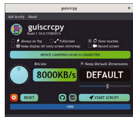
Figure 2: All the functions of the scrcpy command-line tool can be controlled using the guiscrcpy GUI. Click START SCRCPY to initiate the connection.
