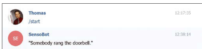
Figure 2: When the delivery person rings the bell, the bot is triggered and my phone vibrates.
