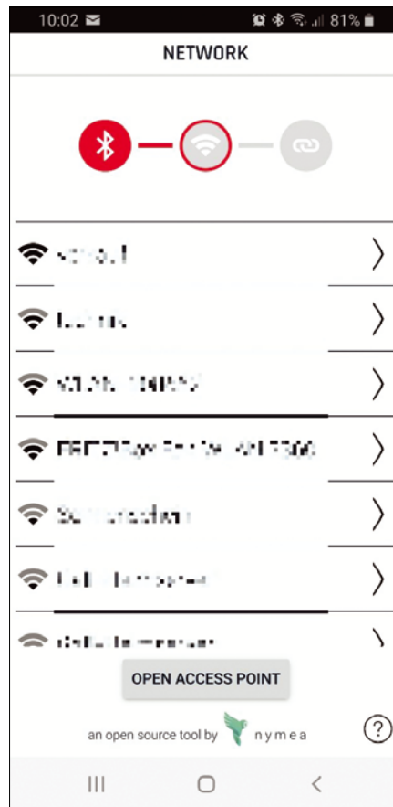
Figure 2: The Raspberry Pi scans the environment for available wireless networks and transfers the list to the BerryLan app on the phone.
