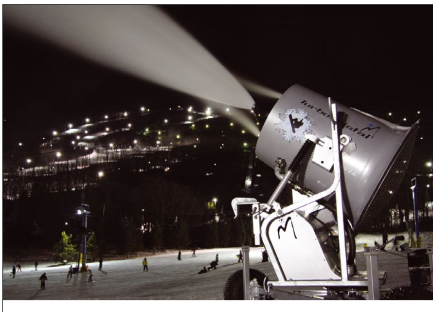
Figure 1: A snow gun makes snow.
