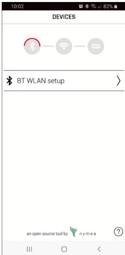
Figure 1: The Raspberry Pi booted with BerryLan shows up in the BerryLan app as BT WLAN setup .
