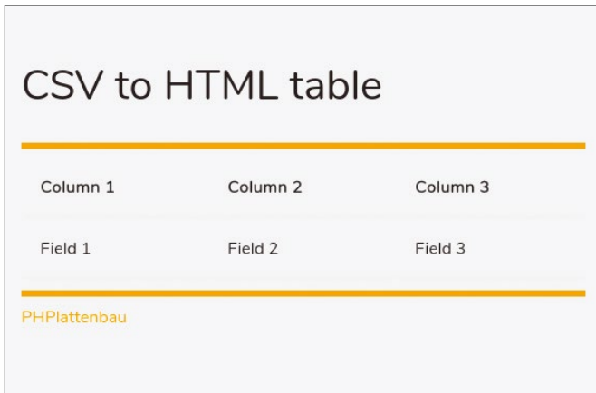
Figure 3: The csv-to-table block lets you use a CSV text file as a simple database back end.
