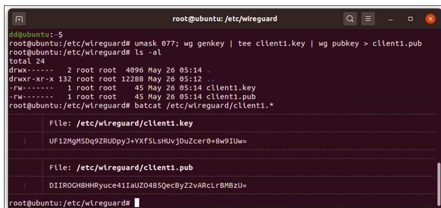
Figure 2: Creating the cryptographic keys is reminiscent of SSH. Repeat the commands on every computer that is involved.
