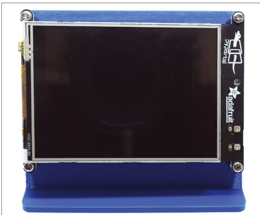
Figure 1: The front of the intelligent PyPortal display. The resistive touchscreen requires a certain amount of pressure before it reacts.
