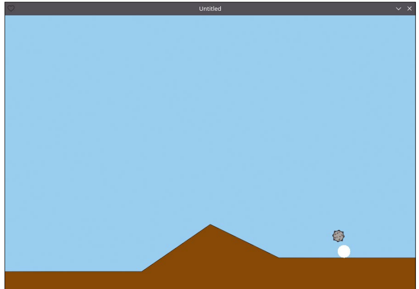
Figure 2: The different points around which the image and the physical body (the white circle) rotate prevent them from lining up.
