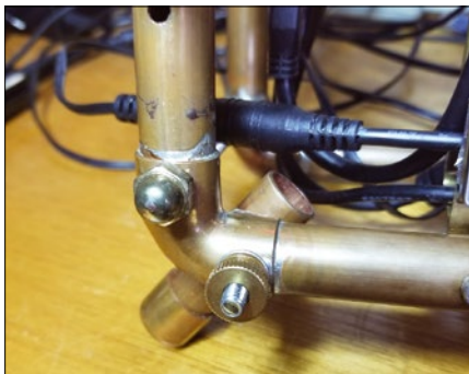
Figure 4: Frame copper elbow corner detail.
