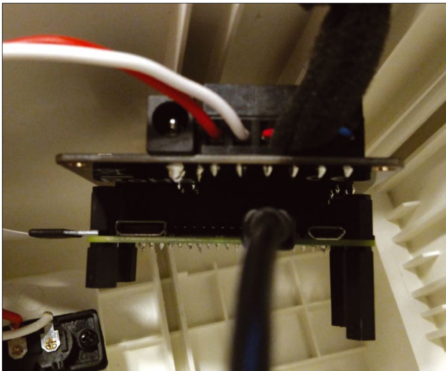
Figure 8: To compensate for a step in the housing, the Raspberry Pi sits on spacers of different heights.
