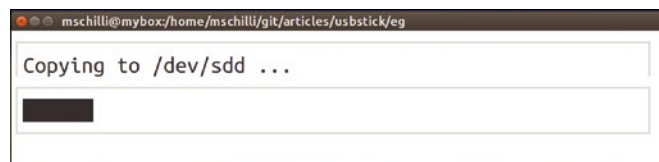
Figure 3: Copying has started. A progress bar shows the number of bytes from the ISO file already copied to the USB stick.
