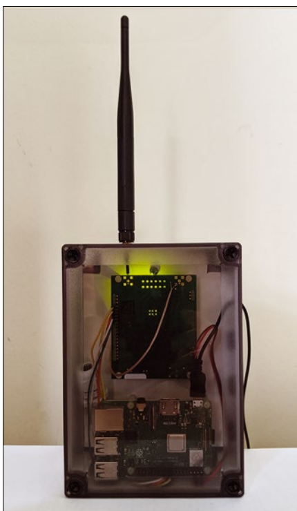
Figure 5: Raspberry Pi and Gateway PCB in a weatherproof box.
