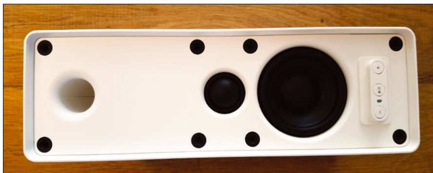
Figure 1: The sound funnel (left), the small tweeter (middle), and the midrange driver (right).
