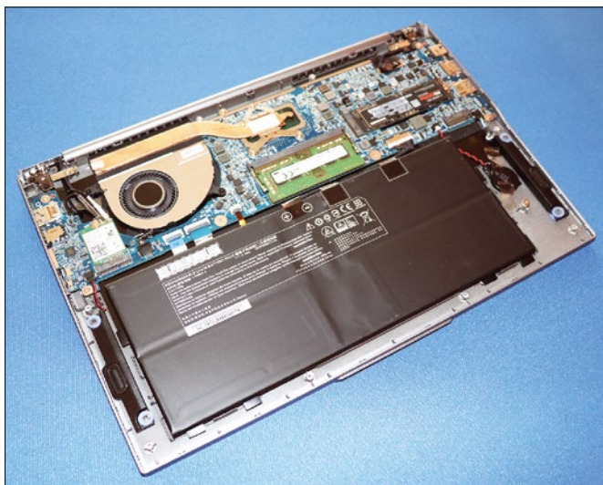
Figure 2: Pop off the back by removing a few screws, and you can swap out the RAM, SSD, and network card.
