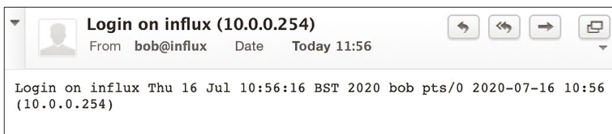
Figure 7: Our simple intrusion detection system notifies by email as soon as a user logs in.
