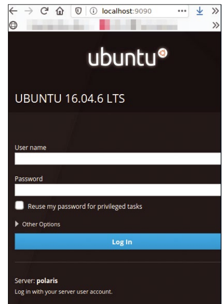
Figure 1: The Cockpit login screen to access the local computer on port 9090. Notice the "Reuse my password ..." checkbox.
