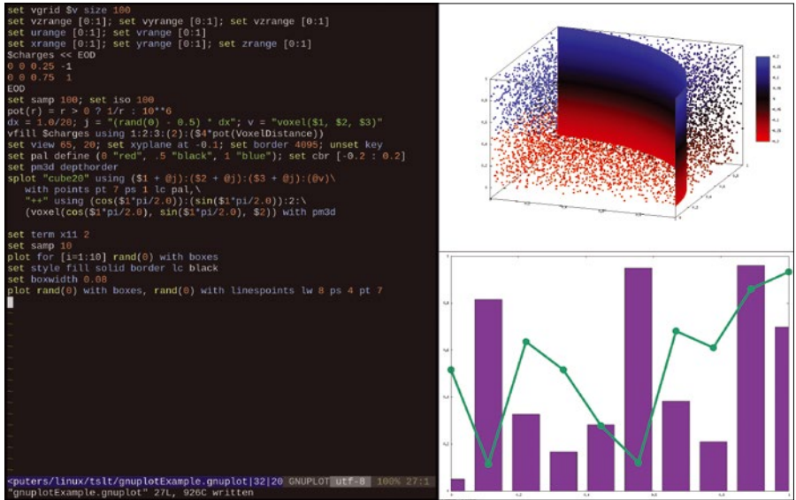
Figure 2: Gnuplot can create all kinds of scientific visualizations. The script on the left created the two plots on the right.
