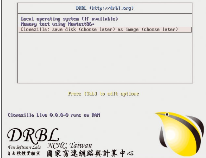
Figure 4: The limited Clonezilla environment broadcast over PXE runs entirely in RAM.
