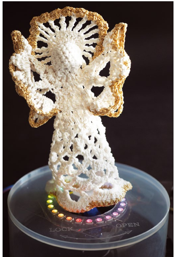
Figure 6: A prototype of the electronic Christmas music box created with a Trinket M0 microcontroller. The capacitive buttons can be operated through the housing.
