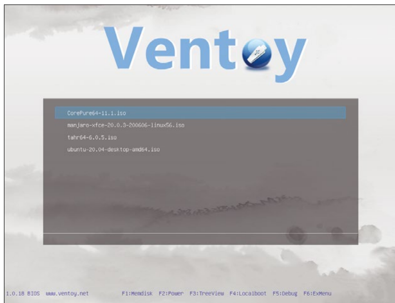
Figure 3: Ventoy in use: We simply used the file manager to copy the Linux images to the Ventoy partition on the USB memory stick.
