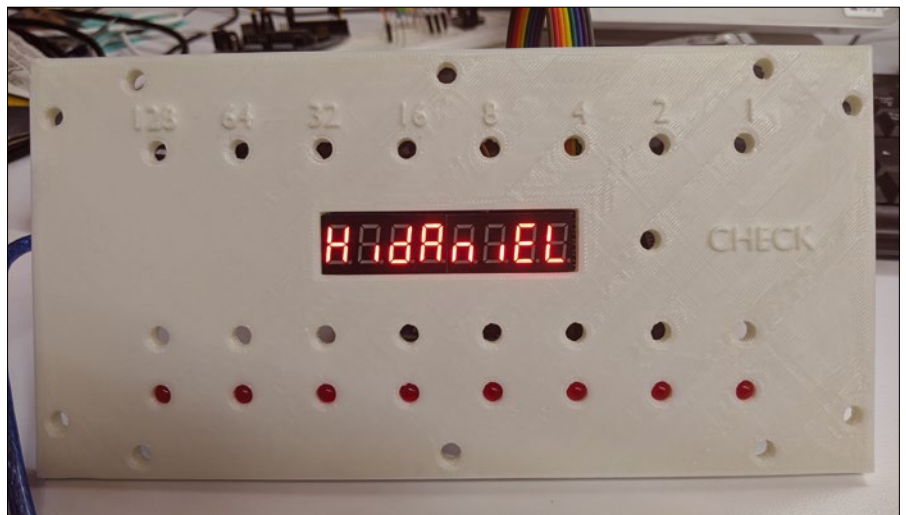
Figure 2: The puzzle faceplate after I installed the LEDs. The empty rows of holes will house bolts as electrical contacts. The holes around the outside are to mount the panel on top of the project box.
