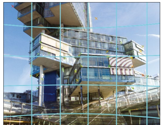
Figure 7: Hugin marks the determined control points in the preview with a colored X.
