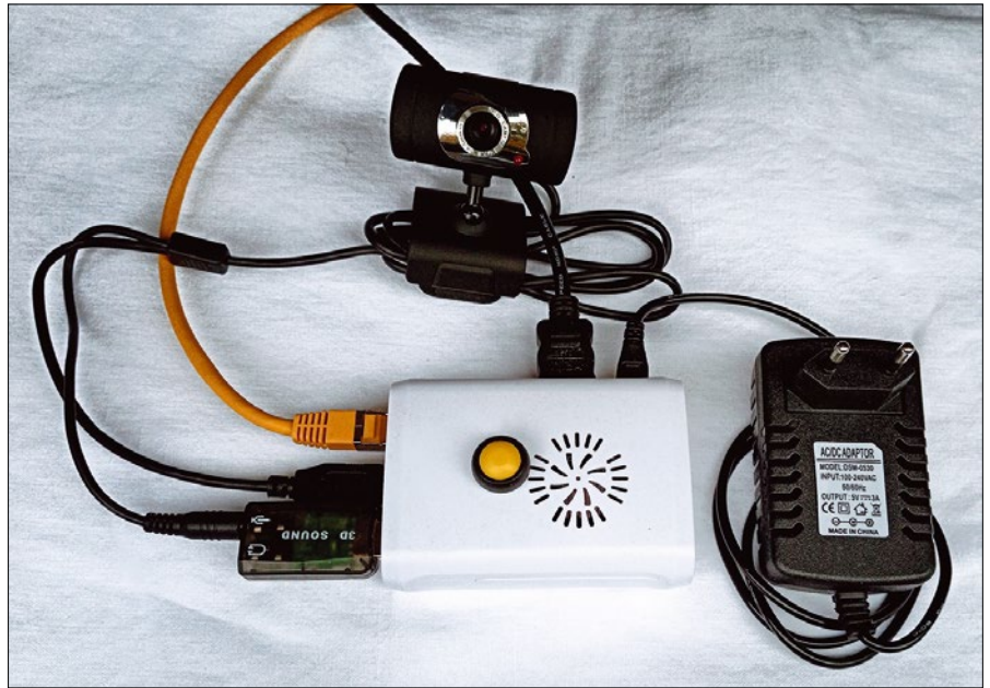
Figure 1: The complete hardware (here with an older webcam and separate USB sound card).
