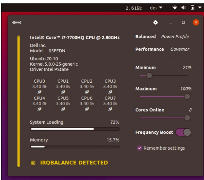
Figure 4: System Monitor and Power Manager for the Gnome Shell shows the clock speed at which the CPU is running and which governor is active.
