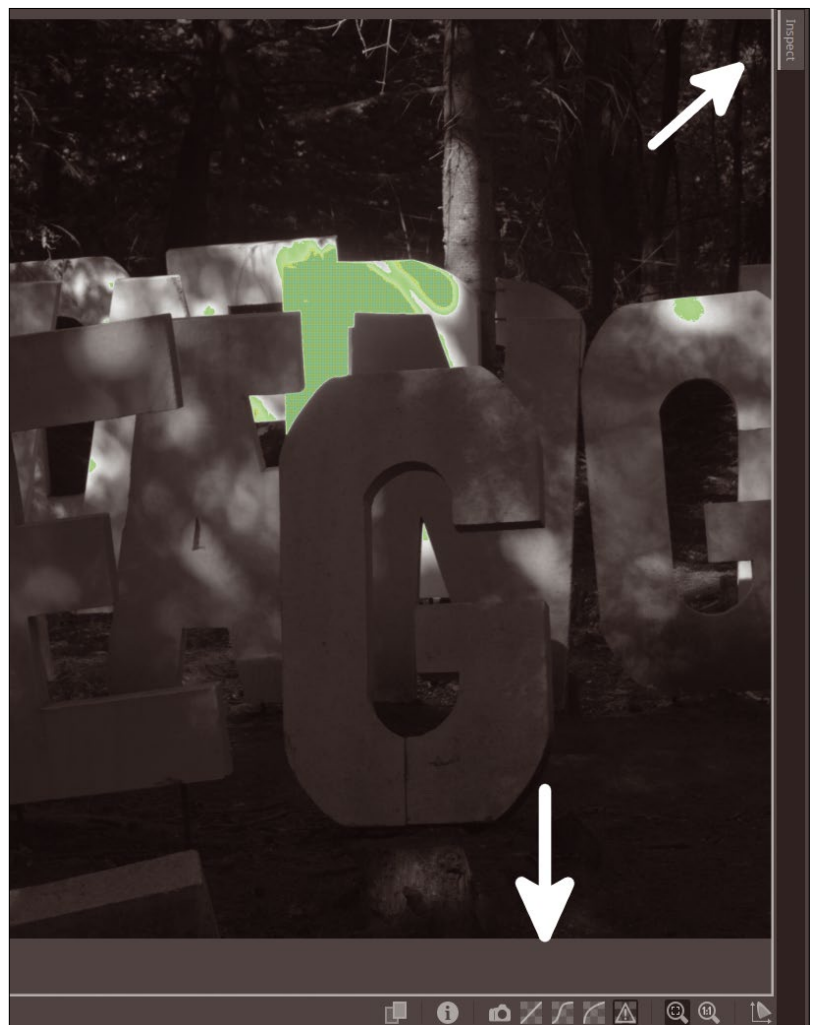
Figure 3: ART offers extensive options for previewing problematic images. In this example, Inspect highlights pixels where clipping occurs.
