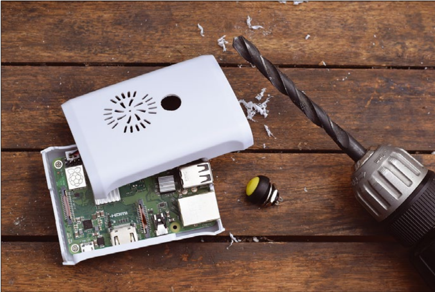
Figure 2: The push button is installed centrally on the top of the housing.
