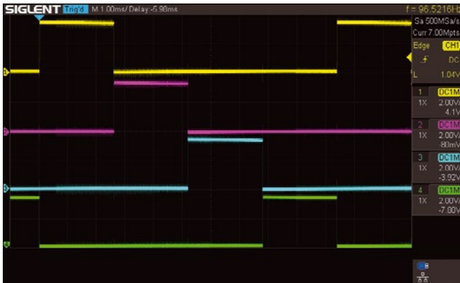
Figure 4: The oscilloscope trace indicates the waveforms produced by gpiomux : yellow = GPIO pin 18, purple = pin 23, blue = pin 24, and green = pin 25.
