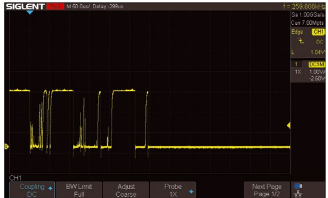
Figure 6: Switch noise – a single press of the switch produces 300ms of noise before settling into the 0 state.
