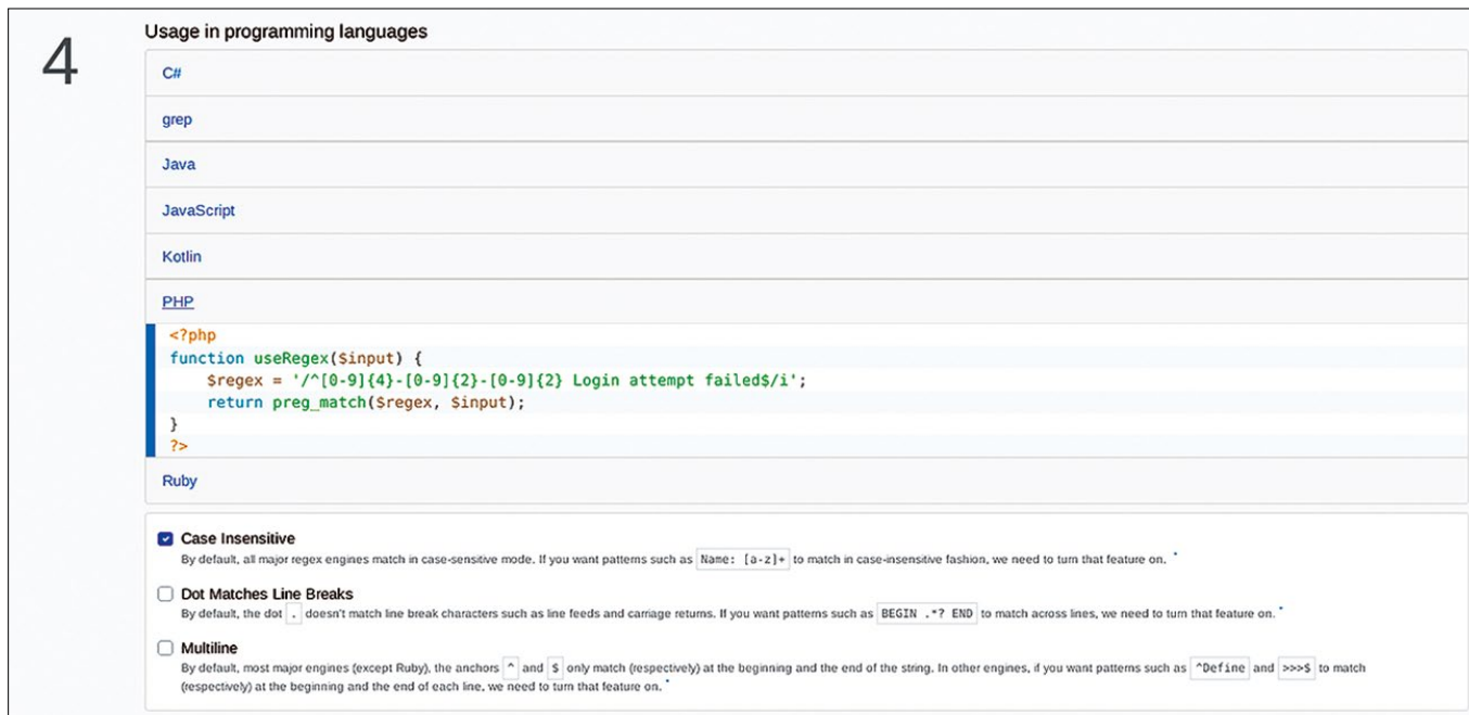
Figure 4: After selecting the desired programming language, Regex Generator displays a regular expression (shown here as a PHP function).
