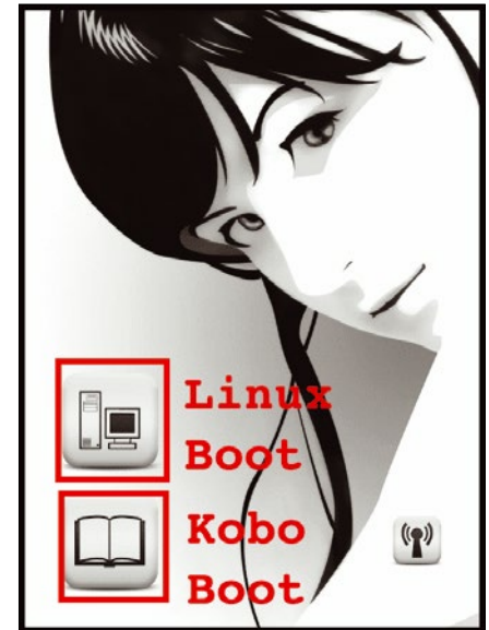
Figure 4: The eReader can now dual-boot to either the original Kobo software or Debian Linux.
