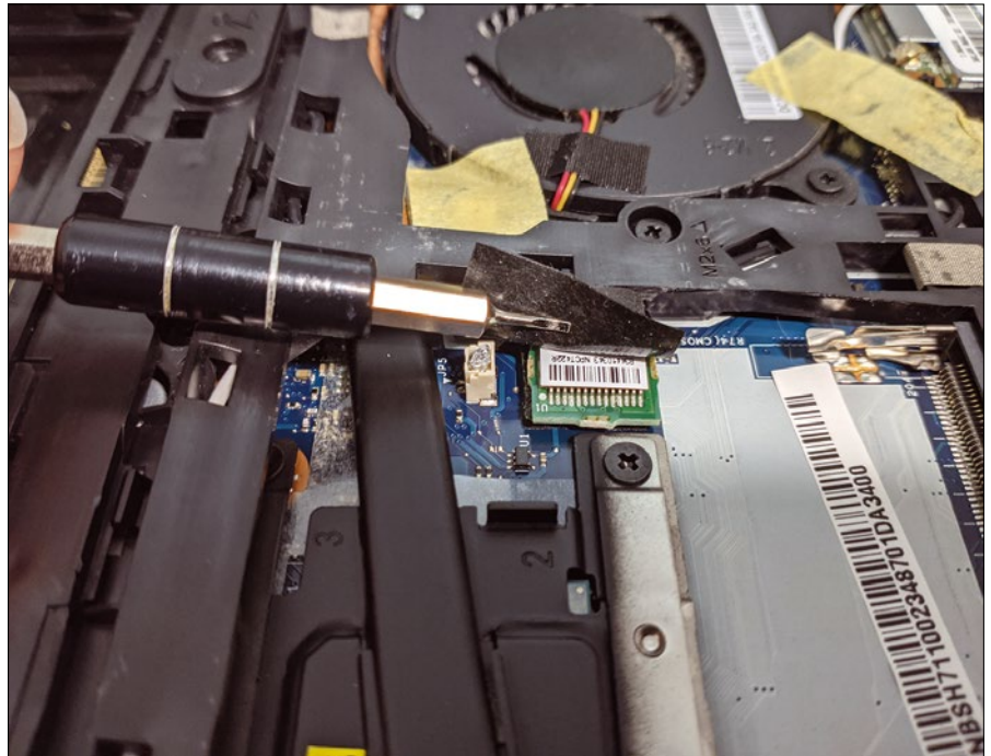
Figure 6: The jumper has already been fitted with an aluminum “rice grain” for bridging.
