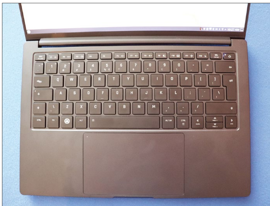
Figure 4: You can configure the machine with many different keyboard layouts. The white dot on the trackpad (top-left) lets you disable the trackpad when typing.
