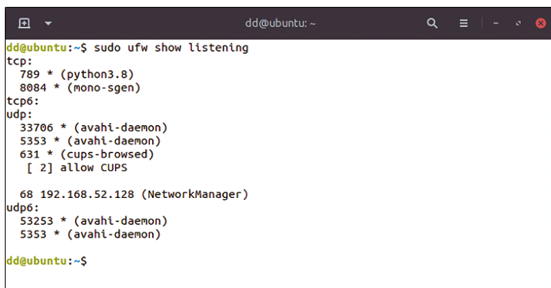
Figure 3: Besides CUPS, the Avahi daemon and NetworkManager also are listening on the network interfaces.
