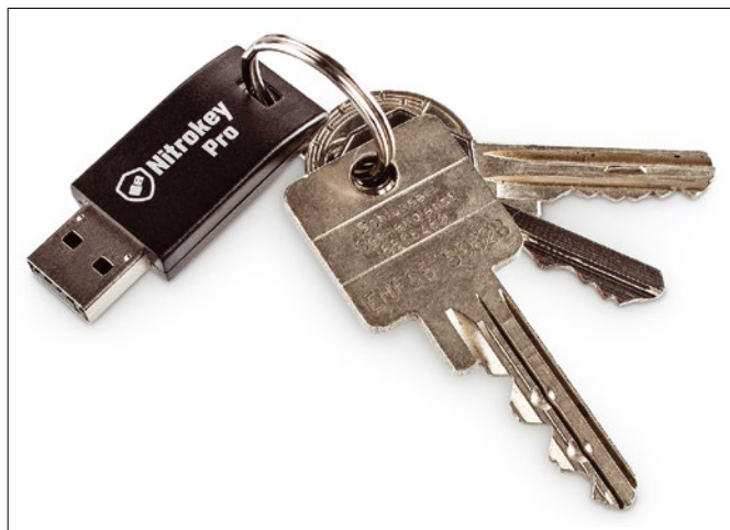
Figure 1: Use the Nitrokey Pro 2 like an OpenPGP smartcard. You can also generate one-time passwords and store access credentials. If you opt for the Nitrokey Storage 2, you will have access to encrypted storage of up to 64GB. © Nitrokey GmbH
