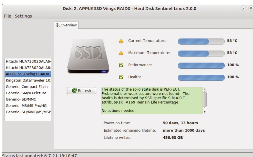
Figure 2: For modern SSD drives, the tool checks how many write cycles the media can potentially handle.
