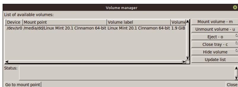
Figure 9: The volume manager controls access to additional filesystems.
