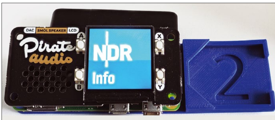
Figure 12: The software can also run on a Pirate Audio HAT by Pimoroni.
