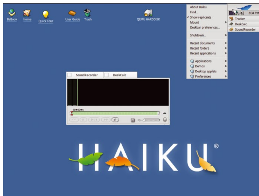
Figure 1: The default Haiku desktop: Note the two apps shown as tabs in the same window and listed in the Tracker on the upper right.
