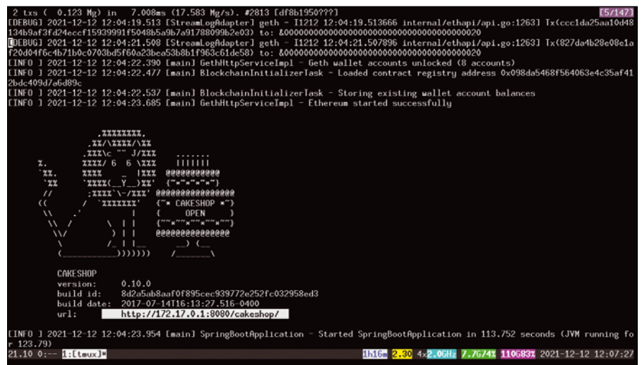
Figure 5: Cakeshop terminal output: The lion with the cake is a marker so that you can see the address to point your browser.
