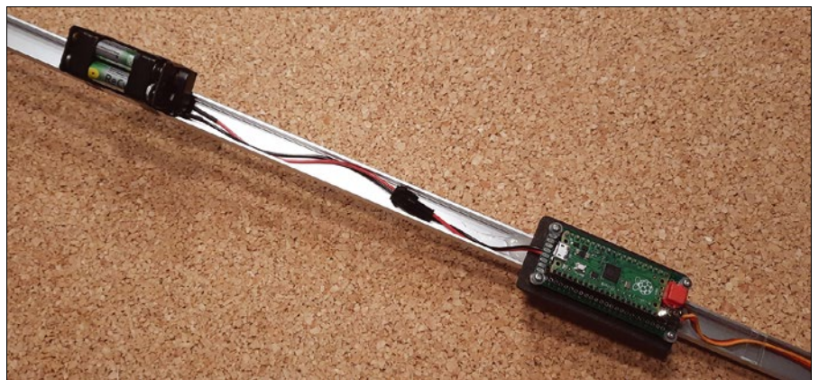
Figure 4: The control board and the batteries are positioned on the back of the light stick.
