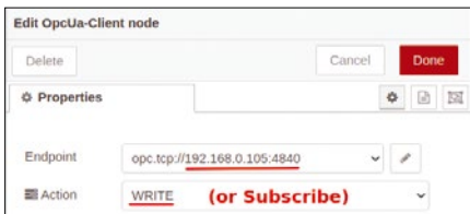
Figure 9: Define an Endpoint and Action for an OpcUa-Client node.
