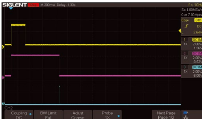
Figure 4: The reset waveforms for the device with a single Set pulse.
