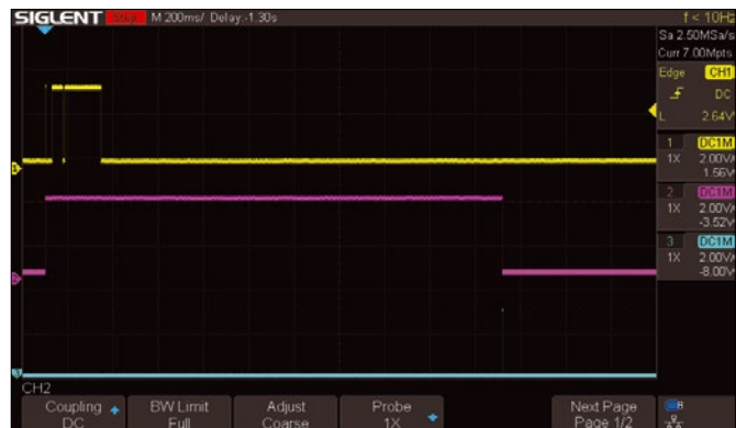
Figure 5: The reset waveforms for the device with a noisy Set pulse.
