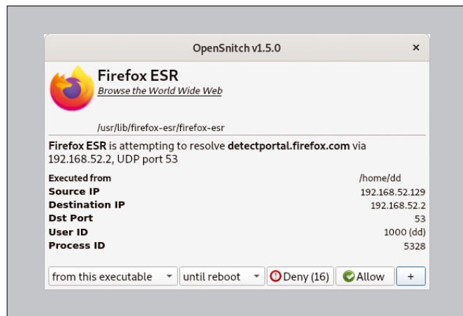
Figure 1: A pop-up window notifies you that Firefox is requesting a connection to update its version. You can allow, deny, or restrict access via various parameters at the bottom of the dialog box.
