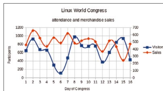
Figure 12: The extra y-axis on the right gives both lines a comparable scale, thus making both of them more readable.
