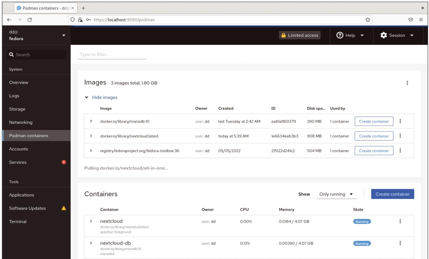
Figure 6: After downloading the images, create the containers that will host the applications.
