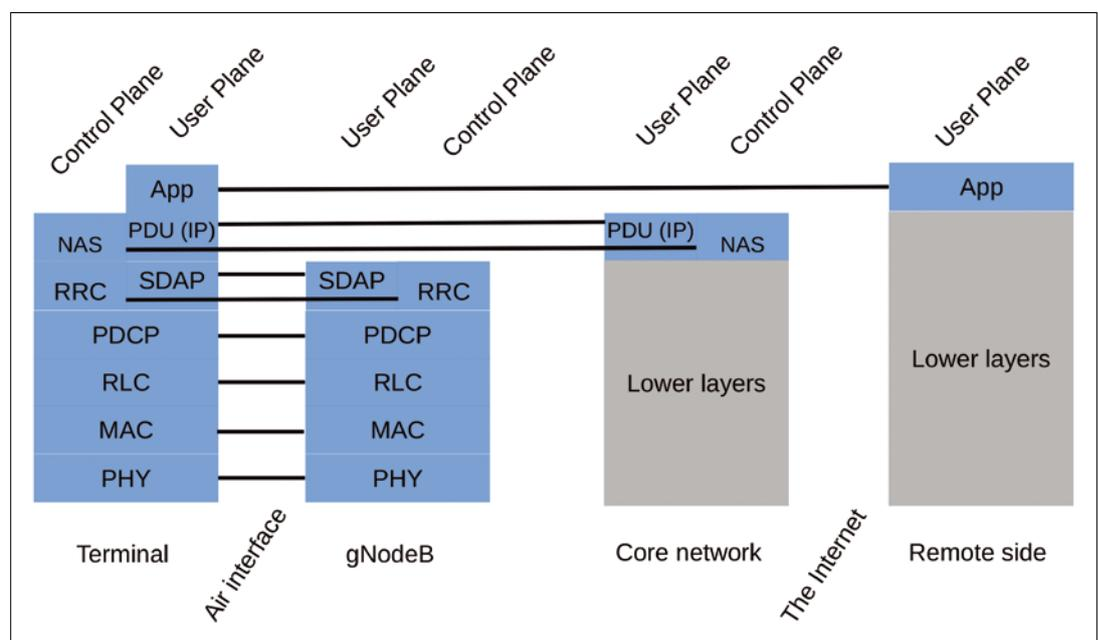
**Figure 5:** Layers of the 5G protocol. Only the interfaces with the terminal are described.
