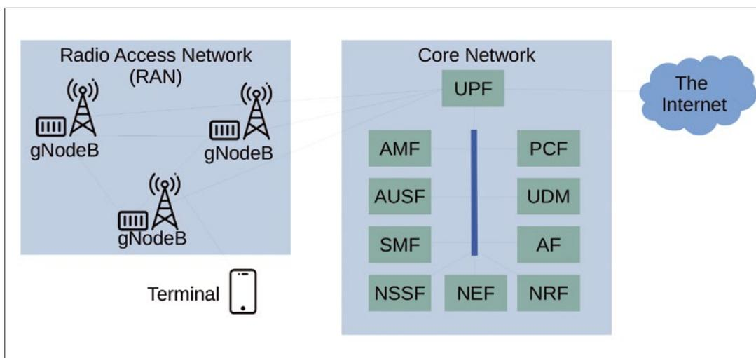
Figure 1: Main elements of a 5G mobile network.
