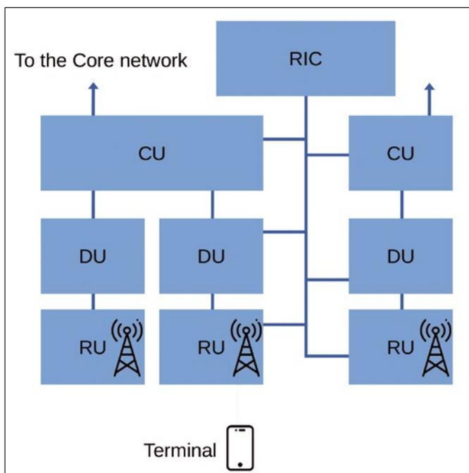
Figure 4: Components of Open RAN.
