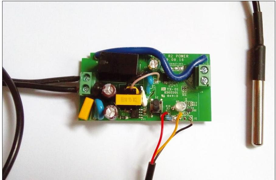
**Figure 1:** The Sonoff Basic WiFi smart switch with temperature sensor.
