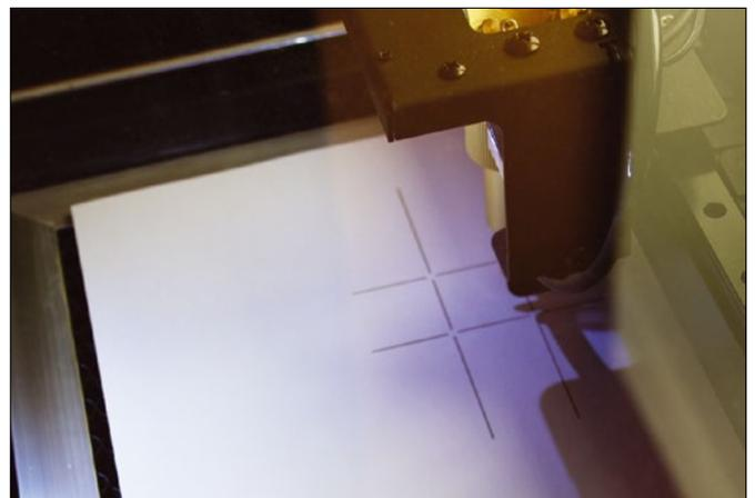
**Figure 4:** Calibrating the FLUX Beamo camera.
