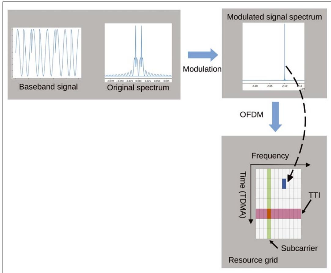
**Figure 6:** Process of modulation/demodulation and the resource grid resulting from TDMA and OFDMA in 5G.
