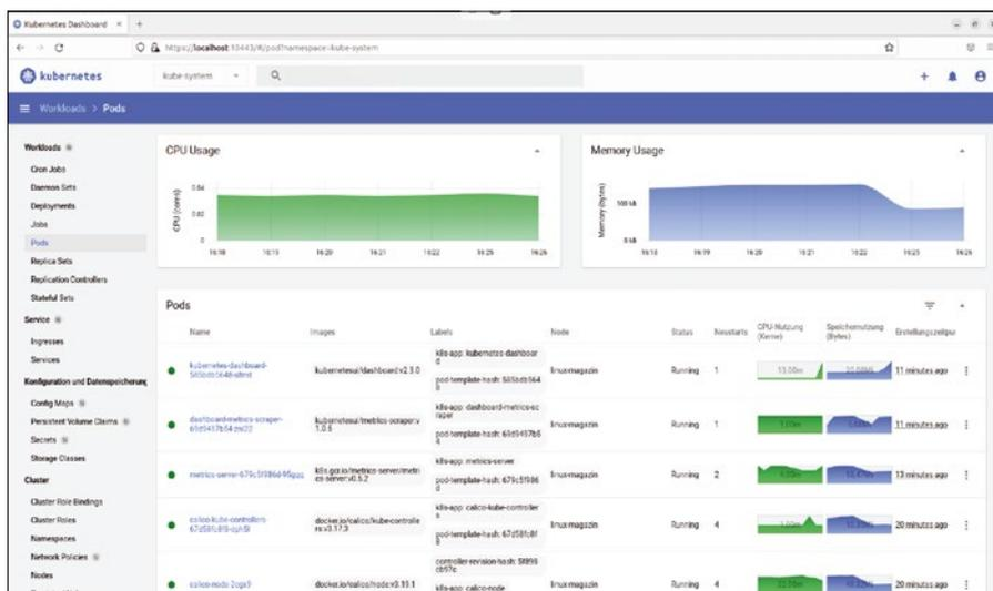
**Figure 3:** A local Kubernetes, including a dashboard, can be set up quite quickly thanks to MicroK8s.
