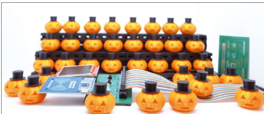
Figure 2: The complete test setup with a horde of pumpkins, the reader at front left, and the display at back left.
