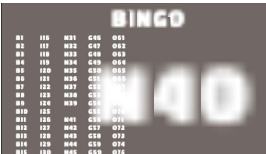
Figure 3: This text was rendered with a pixels-per-unit size of 8. As you can see, the tile number N40 is barely recognizable.
