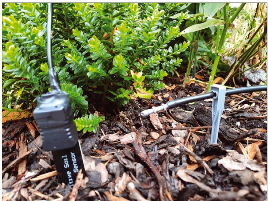
Figure 7: The water outlet and the sensor spike in the plant bed.
