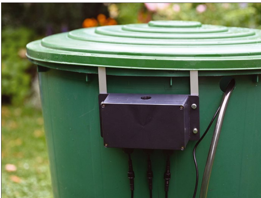
Figure 1: The control unit and supply line assembled on the 200-liter storage tank.
