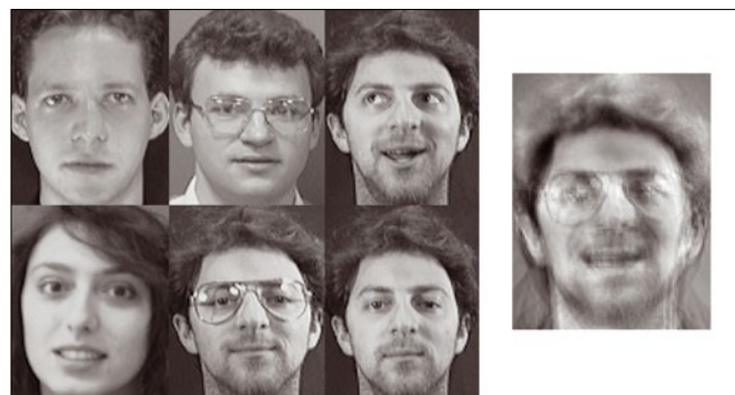
Figure 2: Left: 6 examples of images used for training face recognition. Right: Reconstructed image of a person [4]. © ACM SIGSAC
