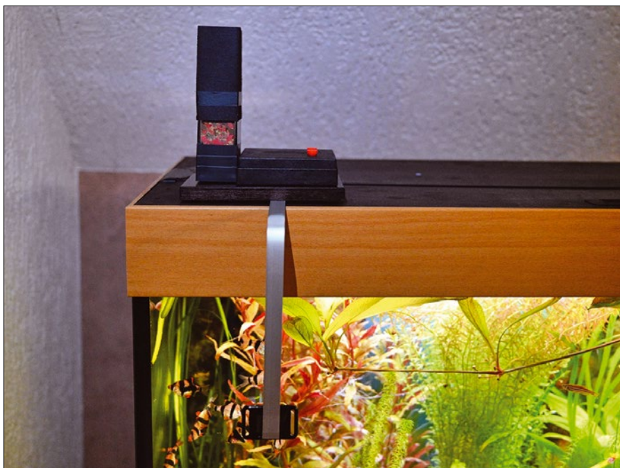
Figure 1: The DIY feeder made with a Raspberry Pi and a camera on the side of the aquarium.
