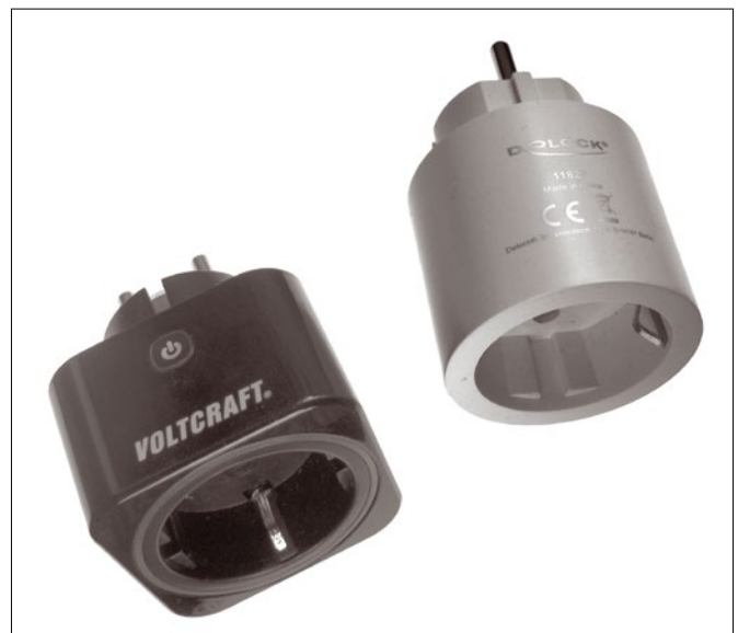
Figure 1: The two plug-in meters used in the test: Voltcraft SEM6000 (left) and Delock 11827 (right).
