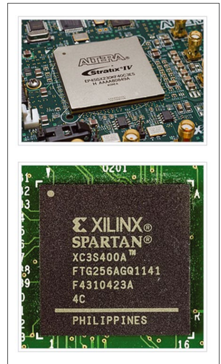
Figure 2: FPGA chips, like the Stratix IV from Altera (top) and the Spartan IV from Xilinx (bottom), can become any digital circuit you want (and run Linux, too).
