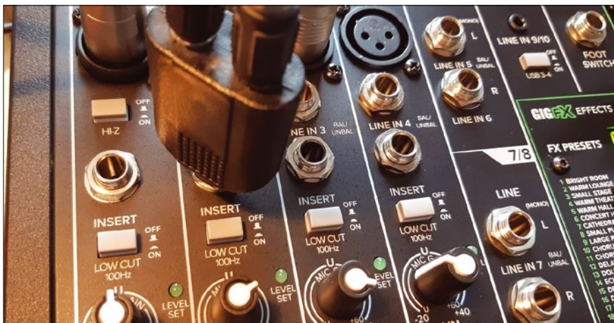
Figure 3: The inserts cannot be controlled; they only loop the signal into the channel. The switch below is responsible for the Low Cut EQ.
