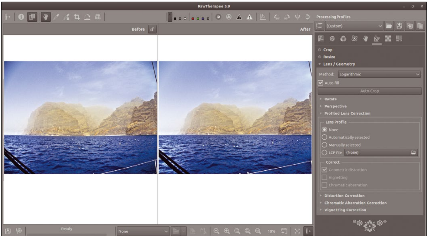
Figure 8: In most cases, distortion and vignetting can be corrected using the Lensfun lens-correction profiles.
