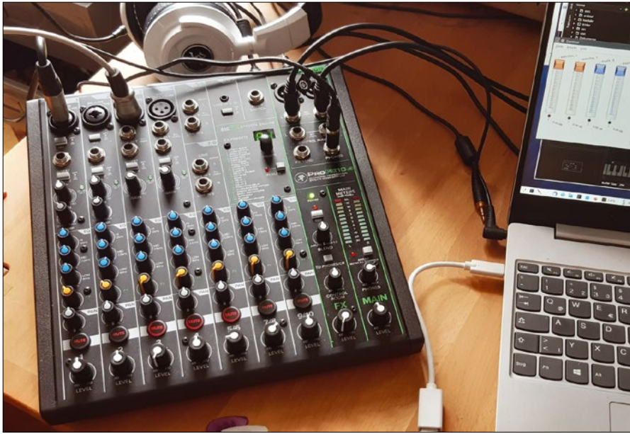
Figure 1: Mackie's ProFX10v3 mixer only has dials instead of channel faders, but it can sit next to a normal laptop on your desk.
