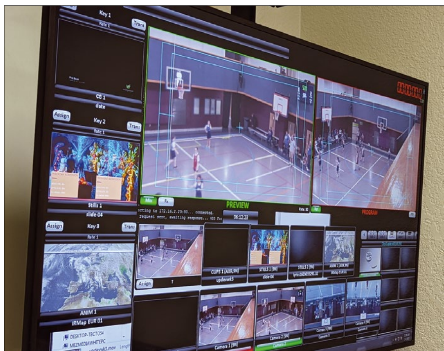
Figure 7: The switcher multiview shows all of the cameras and other sources available. They can be put “on air” by clicking on them.
