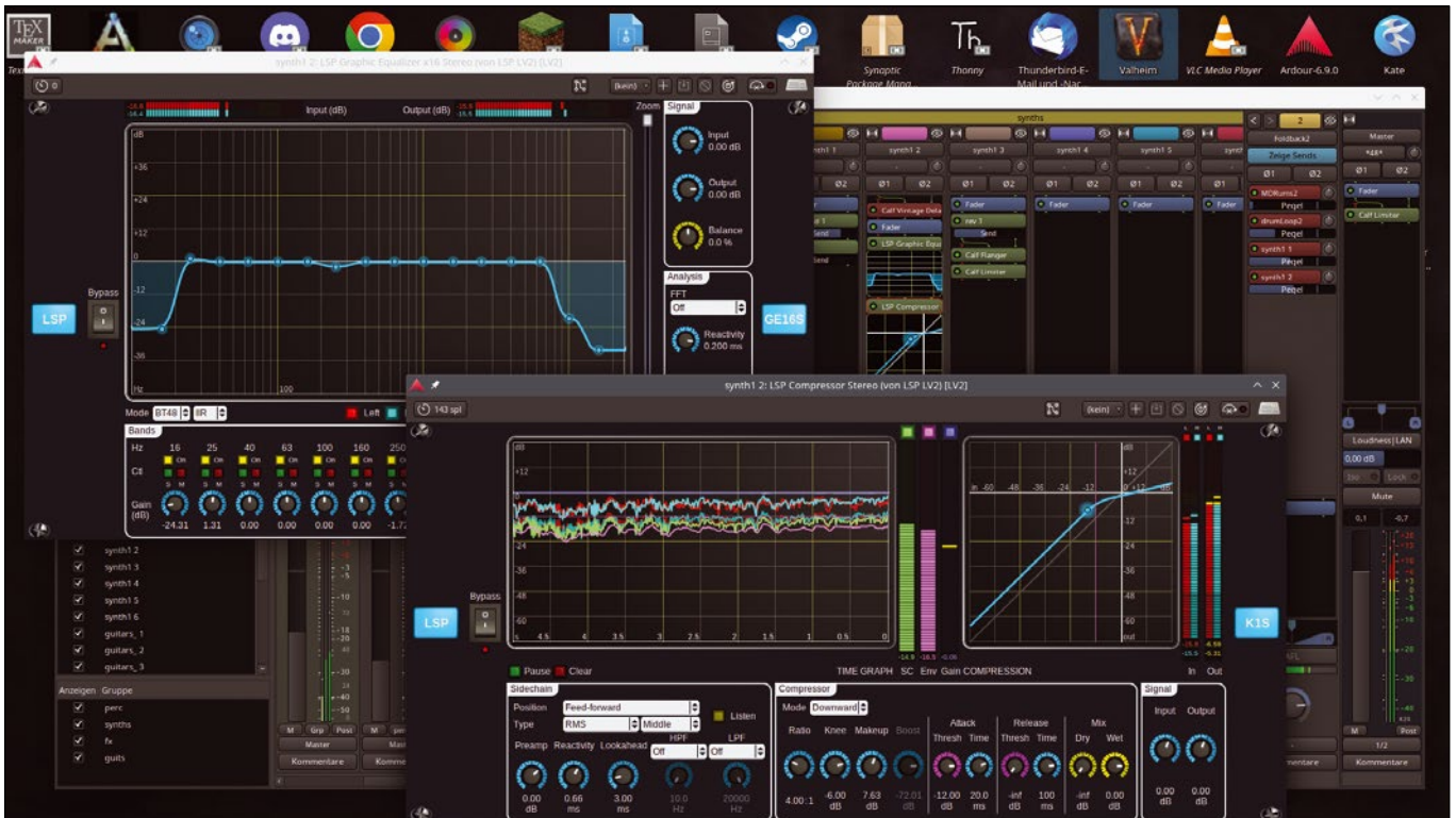
Figure 8: If you are missing any adjustment options in Calf's mastering plugins, take a look at LSP's EQs and dynamics processors. In terms of signal routing, it's hard to imagine more possibilities.
