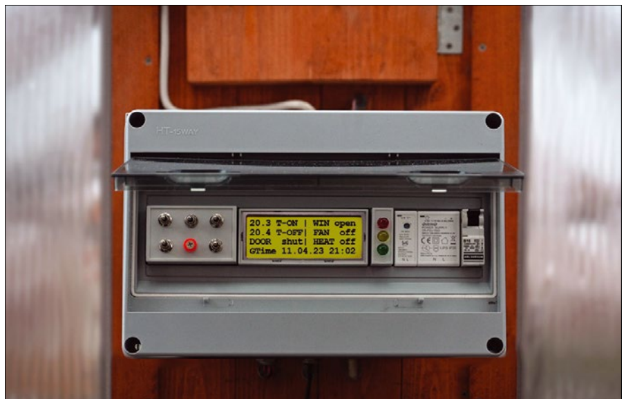
Figure 3: All components are mounted on DIN top-hat rails in a weather-proof housing.
