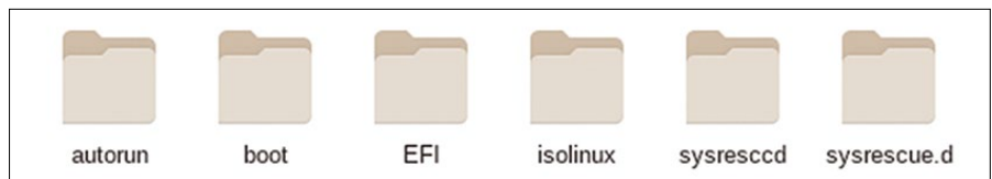
Figure 1: An extracted SystemRescue image: Custom configuration files can be placed under the sysrescue.d directory, and SystemRescueModules under sysresccd .
