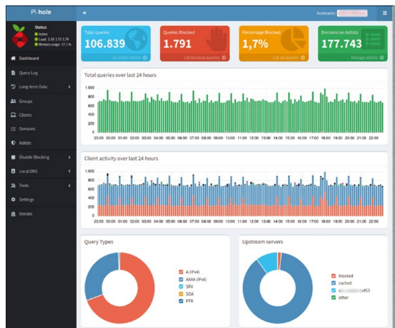
Figure 1: On the fly, Pi-hole filters DNS requests for unwanted URLs and hides advertising content and trackers.
