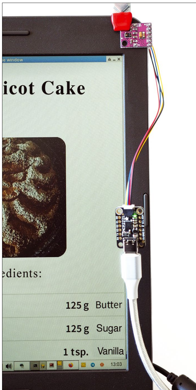
Figure 4: Laptop, MCP2221, and gesture sensor.
