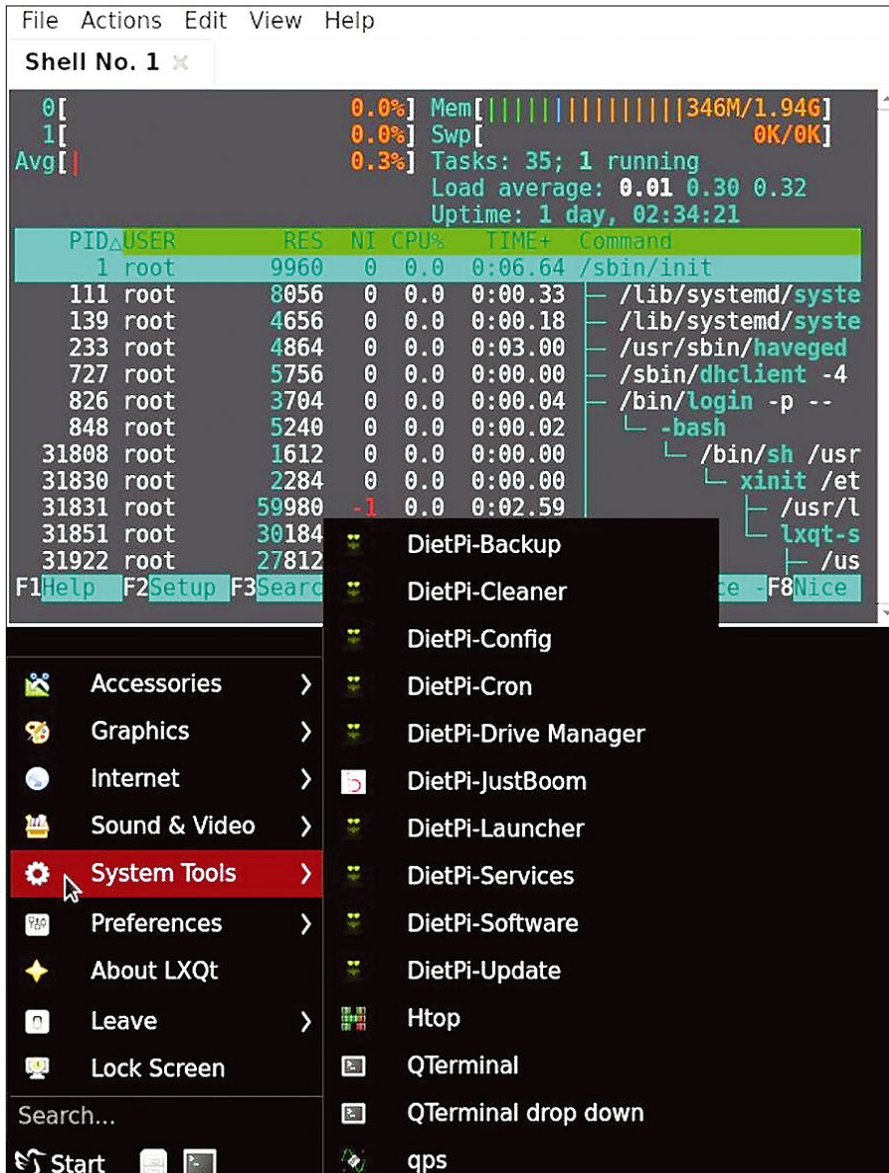
Figure 6: LXQt is just one of the desktop environments offered by DietPi for installation.
