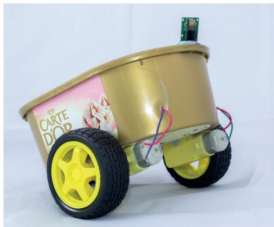
An ice cream tub makes a simple and cheap robot chassis – just make sure you wash it out first.
