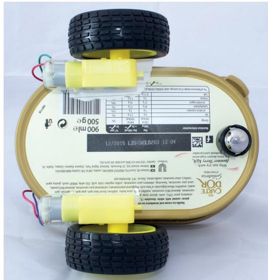
A bit of glue will hold the motors in place, but be careful not to get any on moving parts.
