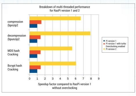
The multithreaded CPU tests were perfect for version 2 to show off its processing power.
