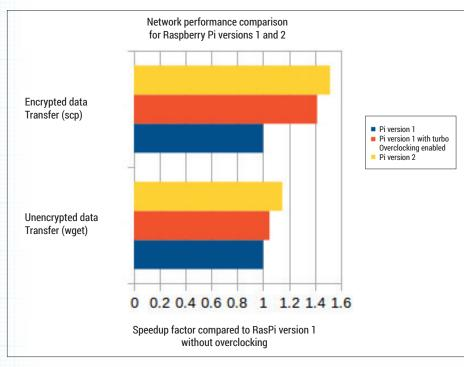
The speedup in encrypted transfer came as a bit of a surprise to us, but is useful for many setups.
