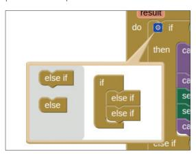
Initially the **if** construction only has one possible condition. You can add more using **else if**, which can be found via the blue cog icon.
