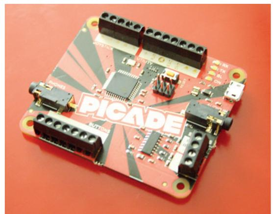
The Picade PCB is an Arduino-compatible board that handles input from the controls and the audio.
