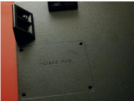
The Picade frame is marked with the positions of major components such as the PCB, Raspberry Pi and controls.
