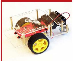
Launched via a successful Kickstarter crowdfunding campaign last year, the GoPiGo turns your Raspberry Pi into a fully functional two-wheeled robot. The \$90 Base Kit includes everything you need – the GoPiGo board, chassis, wheels, motors, encoders, and power battery pack – and is easy to assemble.
