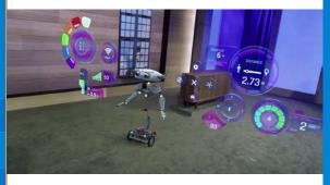
B15 responds to gestures and voice commands, but the virtual portion is only visible through the HoloLens headset. Anyone without a headset will see nothing but the wheeled physical robot body.
