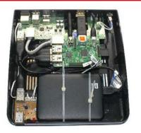
A second generation of the popular MEDIAPI set-top box-style case has been released by SB Components (**sb-components.co.uk**). The MEDIAPI+ features a 3A power supply (with UK, EU, and US plugs) to power the case's 4-port integrated USB hub that routes connectivity to the front and rear. It features IR support and an accompanying IR remote control, as well as space for a USB hard drive. Learn more at: **sb-components.co.uk/products/mediapiplus**
