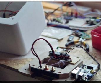
Above The project also uses an Arduino Nano, partly to help reduce the CPU load on the Raspberry Pi, which uses up to 70% on decrypting Spotify tracks
