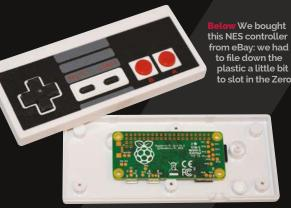
Once all the hardware is complete, you can then set up RetroPie (magpi.cc/1HVgNba) on a microSD card. If you have a spare Raspberry Pi lying around, it might be best to get the initial setup sorted on there first before plugging it into your NES controller to set the buttons. Remember that you only have the buttons which exist on an NES, so make sure any games you put on there don't require more than you have.
