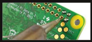
Above Take your time when soldering the pins, and be careful not to connect two or more together with excess solder
