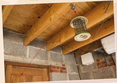
David decided to build a bark-activated automatic door opener. A noise detector circuit is wired to the input of the Raspberry Pi to detect barks. A motor driver circuit drives the actuator that unlocks the door, and a weight and pulley system swings the door open when it's unlocked.
