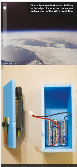
A basic case with the bare essentials needed to make things work, which is important when you're trying to save weight
