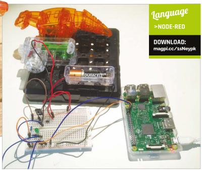
allows higher currents to be switched, and so this circuit can be used for other projects – but never mains or AC. Assemble the dinosaur kit. Make sure the dino can nod freely. The kit's battery holder and motor connect straight to the breadboard. You don't need the switch. On the Raspberry Pi, use the ground on physical pin 39 and GPIO pin 37.
