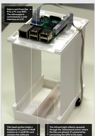
maybe thousands of flies at once because [the ethoscopes] are so small and cheap to maintain," explains Giorgio. "By using the Pis, we have enough computer power to analyse their behaviour using video imaging and we can be wallet-
