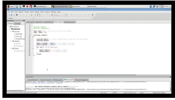
debug mode. It will stop at the red dot, waiting for us to tell it to either continue or to step through the code using the icons next to the red arrow, which provide different step options for the code. More on that later, though. Code::Blocks gives a wide range of tools and functions to help us debug, but if this is your first time running it, not all of them will be visible – we will make them visible as our needs and experience increase.
