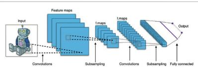
Figure 3 There are many different types of neural networks, specialised for different use cases. For computer vision and natural language processing, the most common type is the convolutional neural network (CNN). It breaks up images into small squares to identify common shapes and features (such as arcs, circles, dots, and lines). It's based on our understanding of the biological cortex. Image credit: Wikimedia
