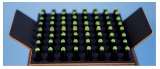
the two coloured vials of the kit in each PCR tube, you create a mixture that emits green when the NeoPixel beneath shines blue.
