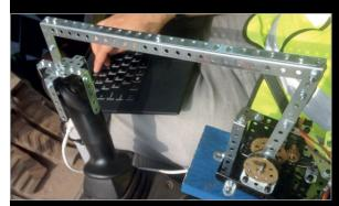
RITH developed "a solution for controlling a full-size digger with a Nod ring," a gestural controller that fits on the finger, for *The Gadget Show*. "We created a simple servo-driven arm controlled by computer to interpret the signals coming from the ring," Sam explains. "The digger arm essentially followed the movement of the user's arm."
