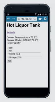
In order to control the temperature, the brewery makes use of three methods – an electronic control panel, a webpage viewable on a smartphone, and a PyQt4 GUI application – all of which can be used at the same time. Fuzzy Duck also uses software running on a Pi for its invoicing and cask tracking. That software was written using Python 2.4 in 2007, well before the Pi's birth, however.
