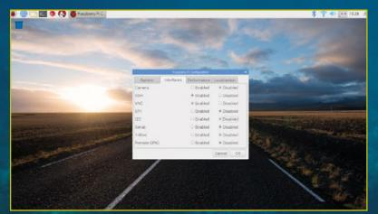
Figure 4 Enable SSH in the Interfaces tab in Raspberry Pi Configuration
