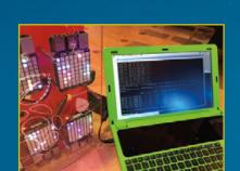
The cluster\_action script is used to control the Raspberry Pi boards
