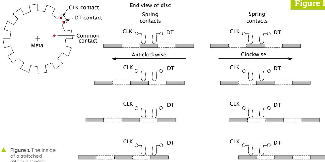
▲ **Figure 1** The inside of a switched rotary encoder
