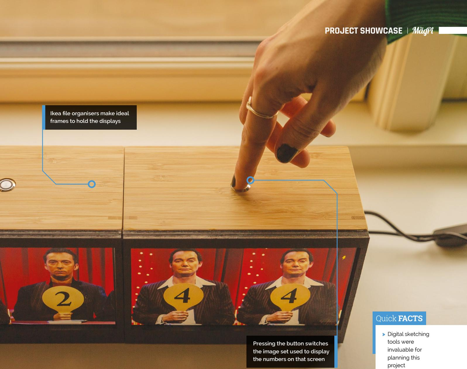
Pressing the button switches the image set used to display the numbers on that screen
