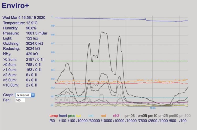
▲ A Flask web server showing real-time and logged data can be viewed remotely from another computer
