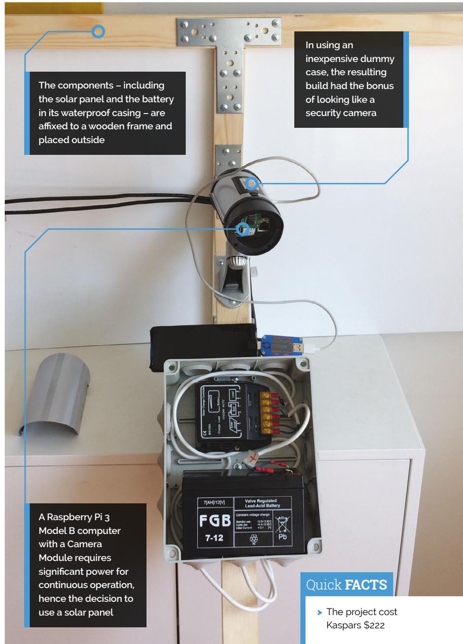
The components – including the solar panel and the battery in its waterproof casing – are affixed to a wooden frame and placed outside
