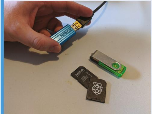
**01** Select a USB stick and plug it into the PiVidBox. As it boots, it detects the USB drive that has been inserted.
