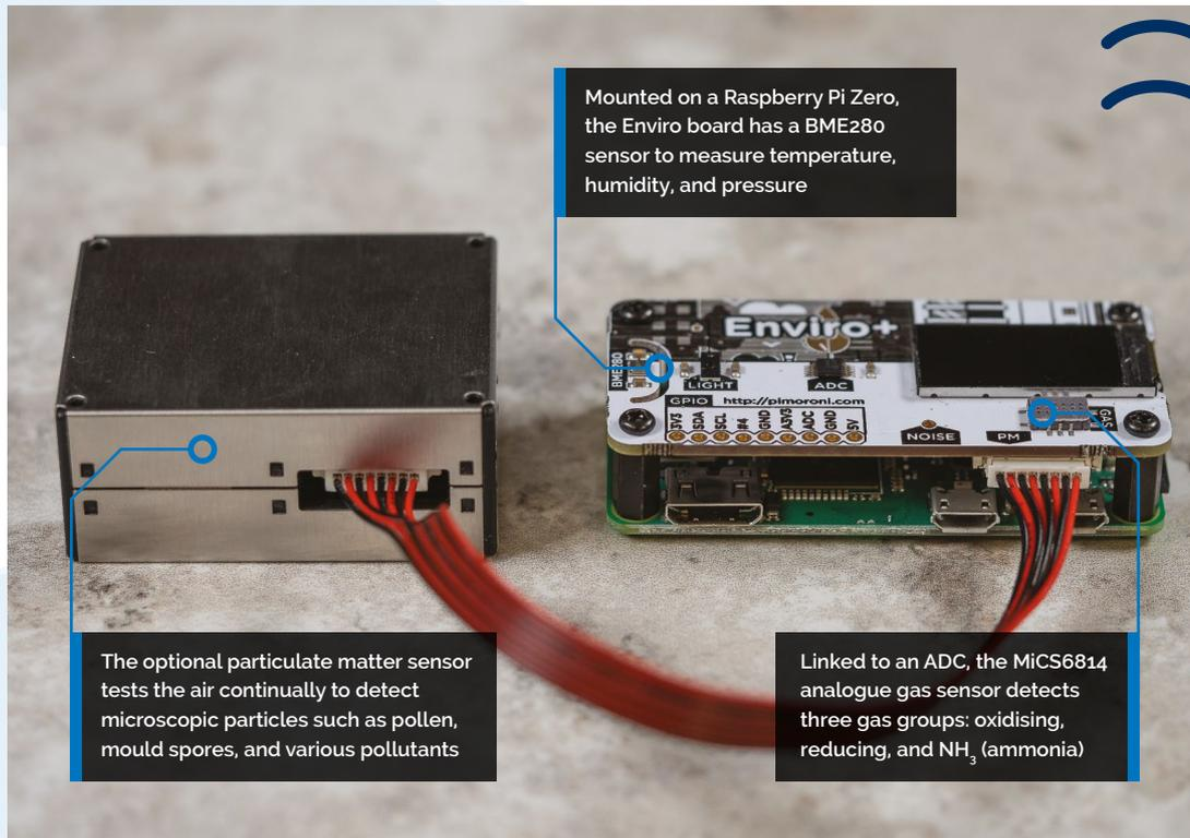
Mounted on a Raspberry Pi Zero, the Enviro board has a BME280 sensor to measure temperature, humidity, and pressure
