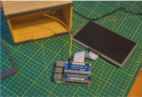
**01** Attach the LCD HAT's ribbon cable to the screen's input port. You might also want to use magnets to help secure the screen in place in its display box. Make sure all the screens are grounded!
