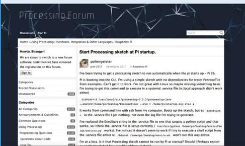
**03** Set the Processing sketch to launch at startup (see [magpi.cc/process](http://magpi.cc/process)). Disable the screensaver (so it doesn't interrupt the clock script) and hide the cursor. Back up the microSD card, then switch on. Repeat steps for the other Raspberry Pi.
