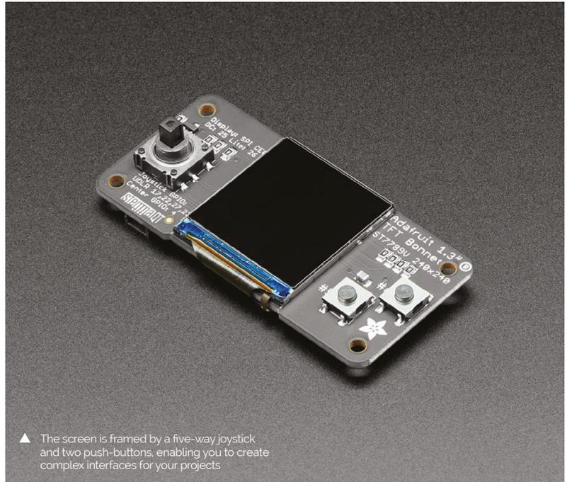
▲ The screen is framed by a five-way joystick and two push-buttons, enabling you to create complex interfaces for your projects
