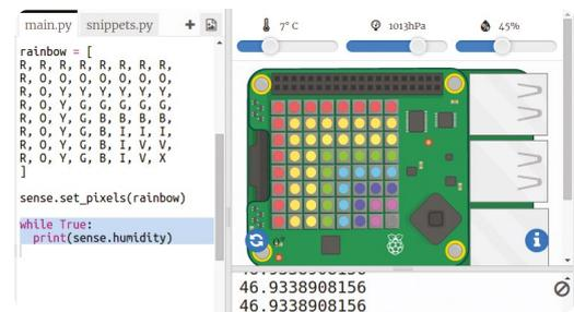
▲ Plot temperature elements as colour values on a Sense HAT's LED matrix. When it displays a rainbow, a real one may well appear in the sky
