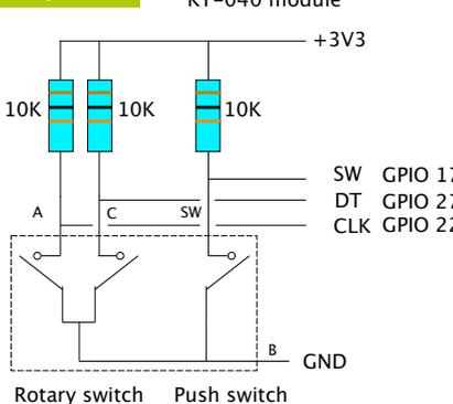
**Figure 2** Schematic of the KY-040 board
