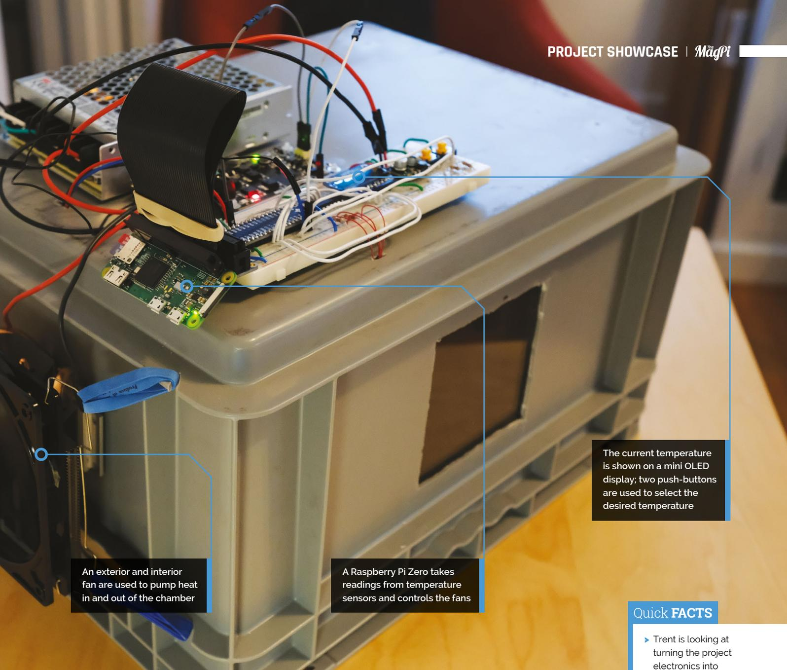
An exterior and interior fan are used to pump heat in and out of the chamber
