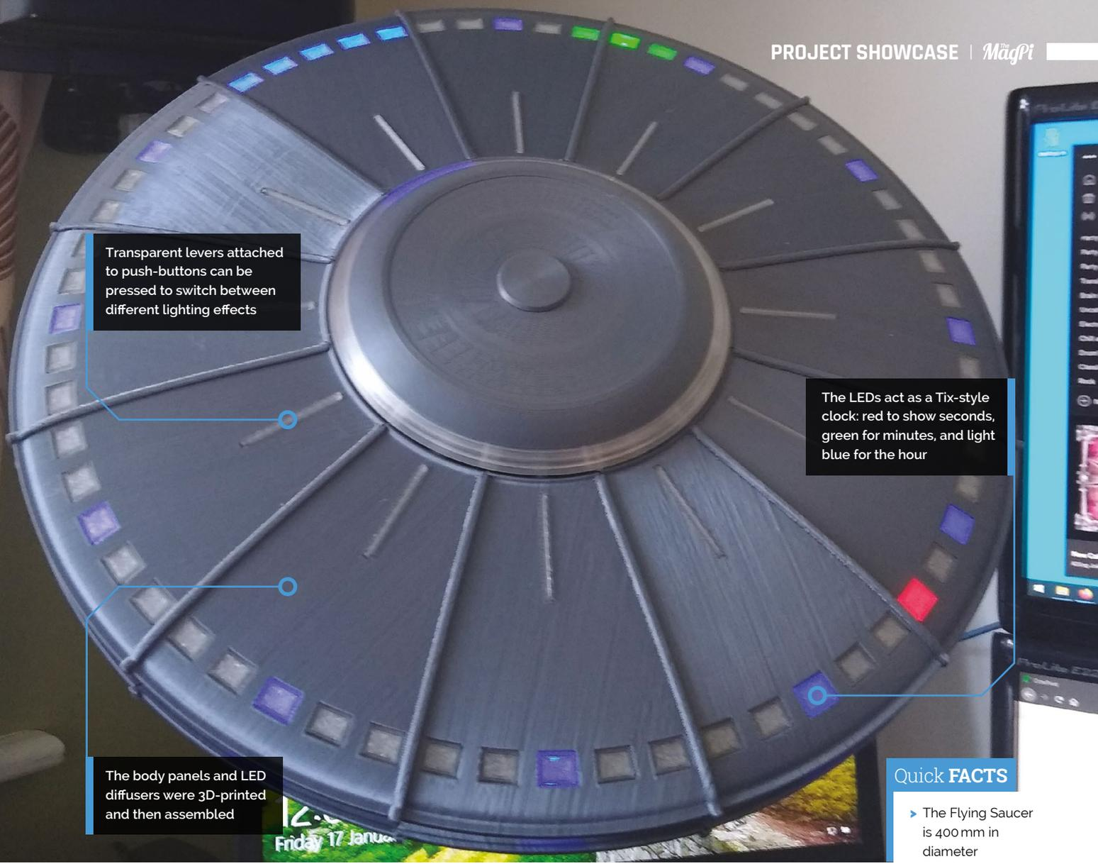
Transparent levers attached to push-buttons can be pressed to switch between different lighting effects
