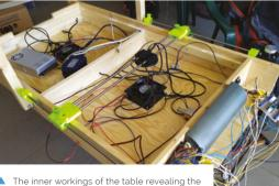
The inner workings of the table revealing to two fans and extensive wiring required After designing the table in Fusion 360, it was constructed from spruce and plywood with an Alubond playing surface. To ensure smooth gliding of the puck, a square mesh of 920 holes was drilled into the game board, enabling air to flow through from two fans located under the table.
