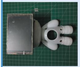
Repurpose or 3D-print a case that will house 01 Raspberry Pi and hold a small touchscreen display in place. Affix the screen to the case.
