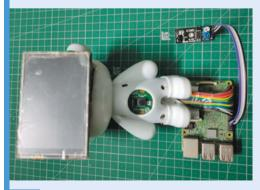
Place an IR sensor on top of the touchscreen 03 and connect it to Raspberry Pi, then screw or clip the rear of the robot shell in place. Use sudoku grids to help train your robot to recognise numerals.
