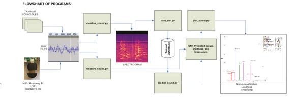
The flowchart explains how the data is analysed by the neural network NOISE POLLUTION MEASUREMENT & CLASSIFICATION USING MACHINE LEARNING ON RASPBERRY PI
