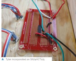
Tyler incorporated an SN74HCT125 integrated circuit to step up the voltage
