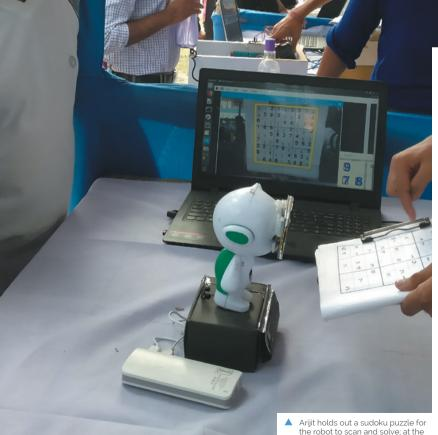
the robot to scan and solve; at the moment, it needs to be held steady robot runs on a Raspberry Pi 3 B+, but he says it could easily run on a Raspberry Pi Zero.
