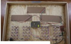
The back end of the project shows the neat positioning of the LEDs connected to a Raspberry Pi Zero W
