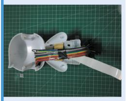
Create a hole for a Camera Module and 02 position it in place. Use jumper wires to connect the screen to your Raspberry Pi.
